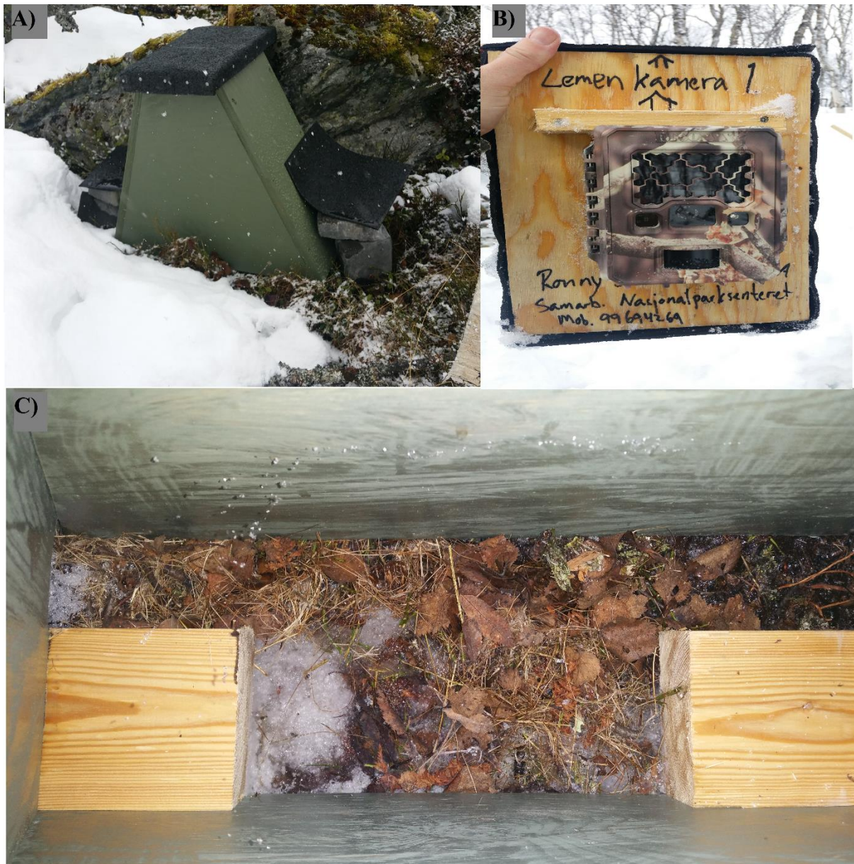
Figure 5: (A) The trap box from the outside. Entry-and exit-points on either side of the box. (B) The trap box photographed opened. The lid of the box with the camera attached. (C) The box photographed from inside. The wooden squares guide the animals in front of the PIR-sensor of the camera.
