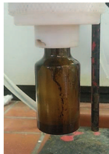
Figure 4-23. Pyrolysis oil collected from the ESP during pyrolysis of milled beech wood in molten salts.
