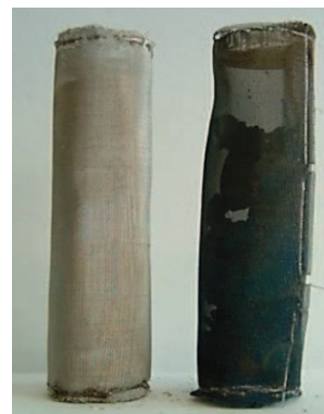
Figure 4-3. Artificial wire-mesh cylinder (d = 14 mm) before (left) and after (right) pyrolysis in a fluidized sand bed (500 °C)
