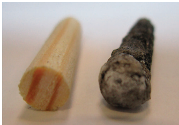
Figure 2. 6 mm pine wood cylinder before (left) and after (right) pyrolysis in FLiNaK at 500 °C. The solid residue is covered and infiltrated with salt.
