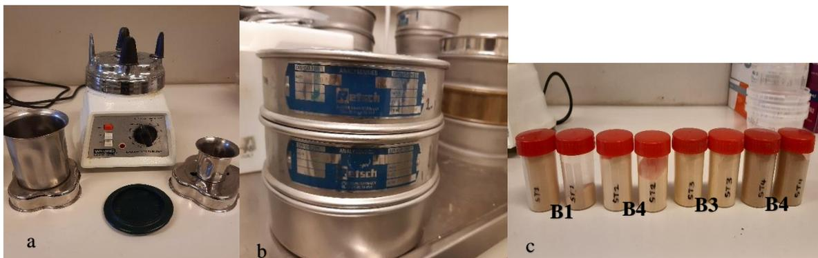
**Fig. 2:** Milling equipment: a= Blender, b= Sieve, c= Samples
