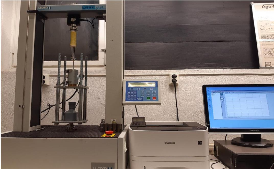
**Fig.6** Pelleting unit connected to Lloyd LR5K texture analyser and computer
