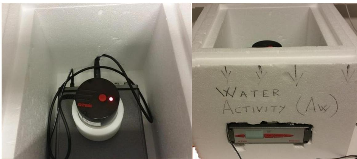
**Fig.7** water activity testing instrument, Rotronic Hygrolab
