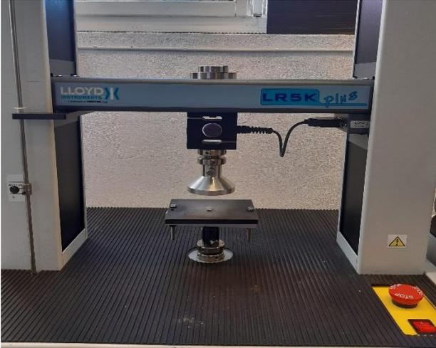
**Fig.8** hardness test instrument (Lloyd LR5K texture analyser)
