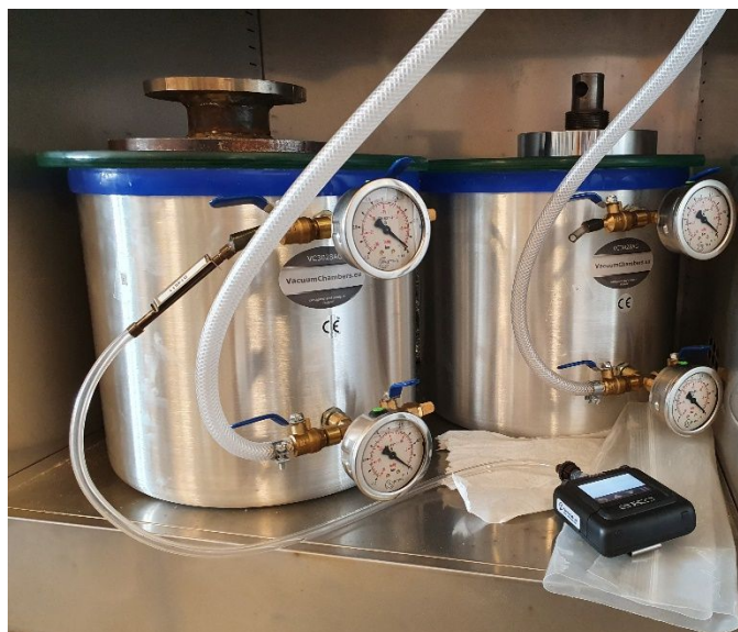
Figure 6: The VOC chambers and an air pump inside the climate cabinet
