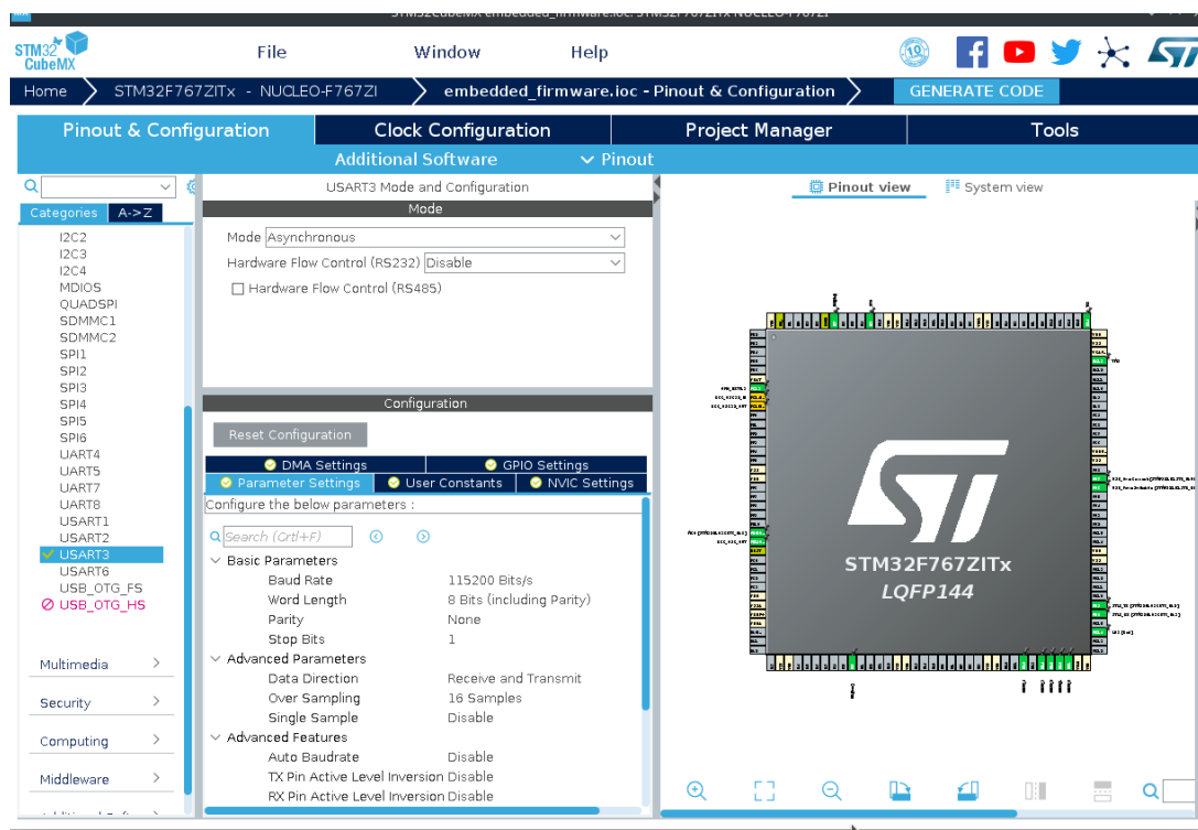
Figure 15: Example of using STM32CubeMX for configuring the UART peripheral on the STM32F767zi. Made by the author.
