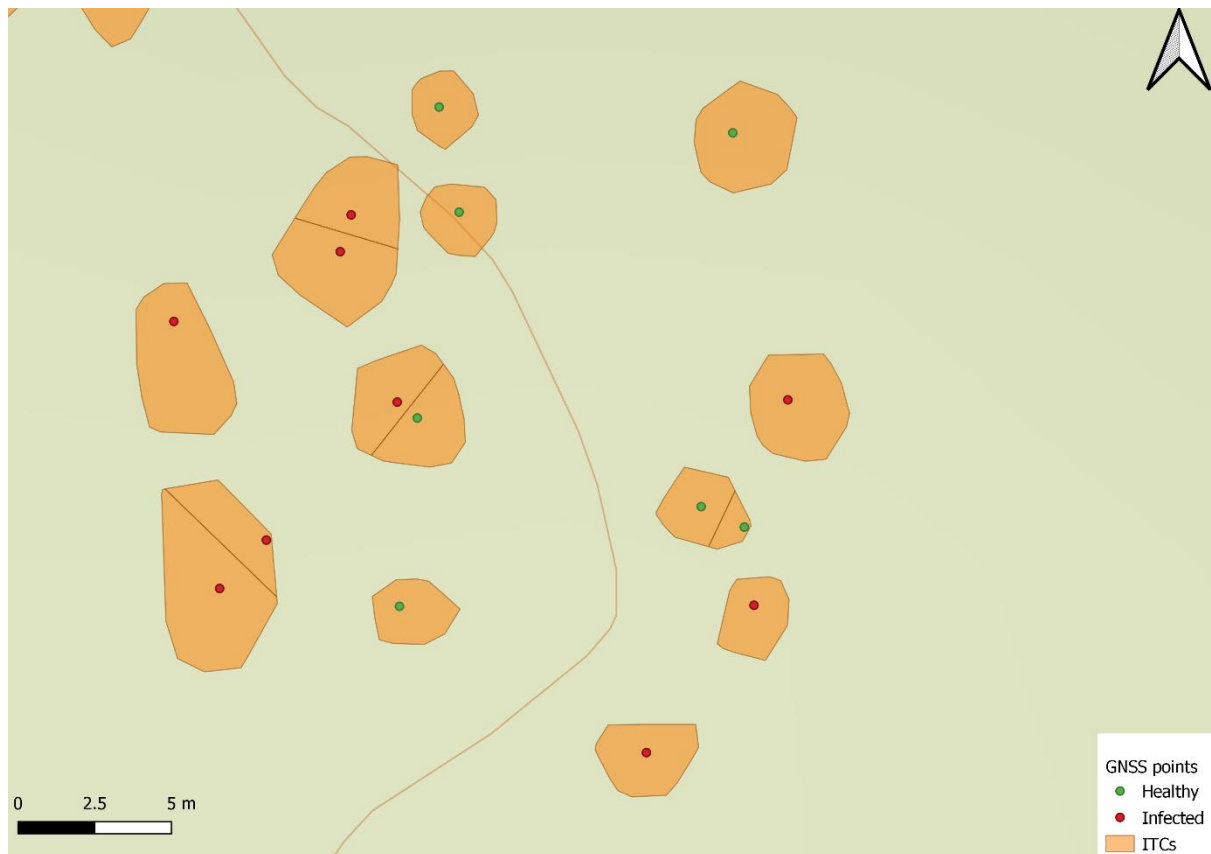
Figure 7: Split ITC polygons as a result of the Voronoi diagram.
