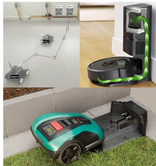
Figure 4-1: Illustrations of robots docking. Top left: WiFiBot QR docking. Top right: Roomba i7+. Bottom: Bosch Indego 350.
