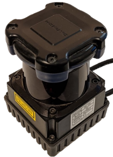
Figure 11-2: An illustration of the Hokuyo UTM-30LX-EW laser rangefinder.
