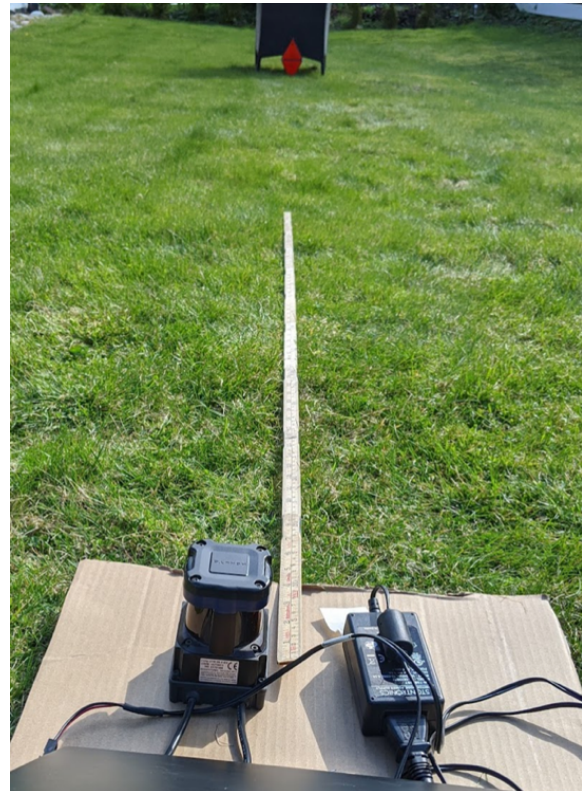
Figure 17-1: An image of the experimental set-up for a range experiment with the Hokuyo laser. The laser is directly exposed to sunlight.
