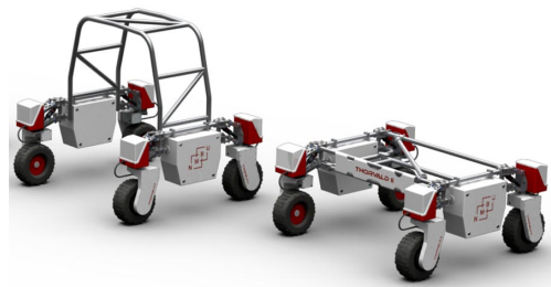
Figure 1-2: An illustration that shows two different configurations of Thorvald II (nmbu.no).
