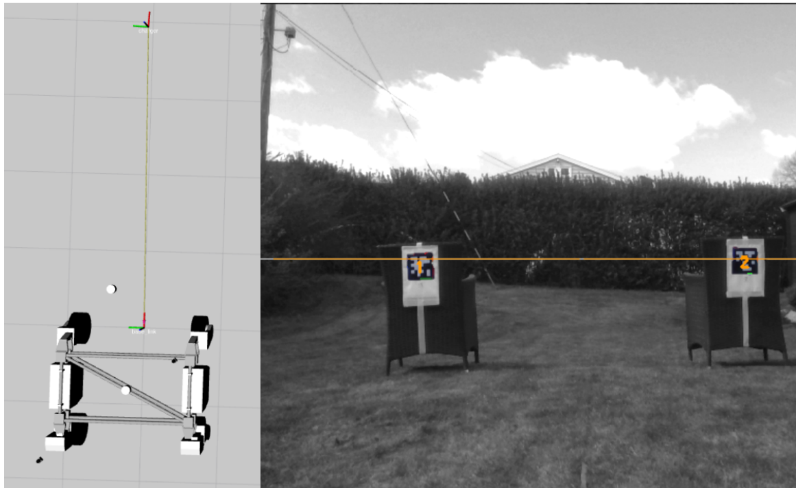
Figure 9-15: An image showing test results from one of the tests, where the AprilTags are detected and marked with their respective ID (1 and 2). To the left is a figure from RViz showing a transformation that was broadcasted to visualize how the charger pose can be determined from the AprilTag detection data.
