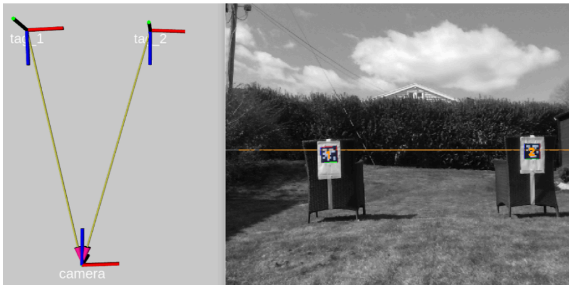
Figure 9-13: An illustration of an accurate and precise result from the test where, in the left illustration, the lower frame depicts the camera frame, and the two upper frames depict the frames of the detected tags. The detector successfully managed to estimate the pose of the two tags.
