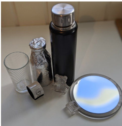
Figure 9-3: An overview of the objects used for a small-scale experiment with the Hokuyo scanner. From left: Water glass, reflective band, bottle covered with aluminum foil, bear-shaped reflective figure, black thermos, mirror.
