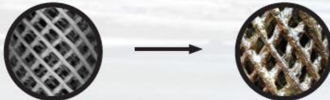
The picture shows the clean carrier material and the growth of biofilm.
