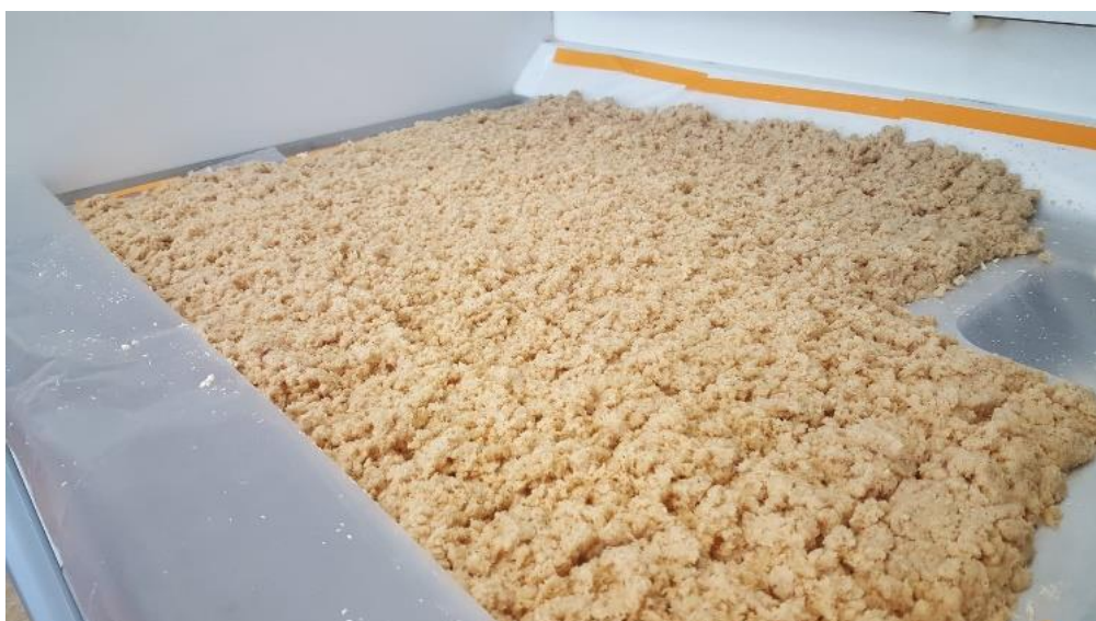
Figure 2.3: Picture of substrate after being spread out on a plastic sheet in a fume hood and left to dry.
