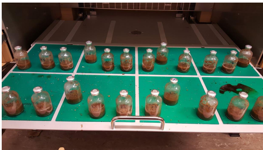
Figure 2.5: 50ml bottles with substrate, buffer, dH 2 O and NaOH. In this picture, all bottles have been preheated and mixed from 15 minutes at 50°C and are ready for enzyme addition to start the hydrolysis reaction.
