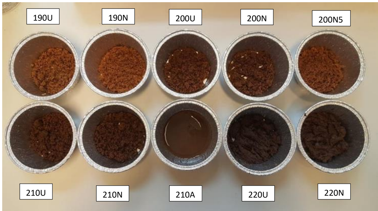
Figure 3.2: Picture of steam exploded spruce. The different samples were added to cups to show how the appearance of treated samples after steam explosion. Note how the high moisture content in the acid-hydrolysed sample (210A).
