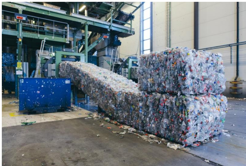
Figure 6 Infinitum sorts plastic bottles by colours and bales the plastic bottles.
