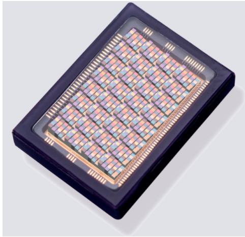
Figure 10: Snapshot mosaic CMV2K-SM5x5-NIR sensor (25 channels, 600 - 900 nm) of Photonfocus AG's camera MV1-D2048x1088-HS02-96-G2, source: [88].
