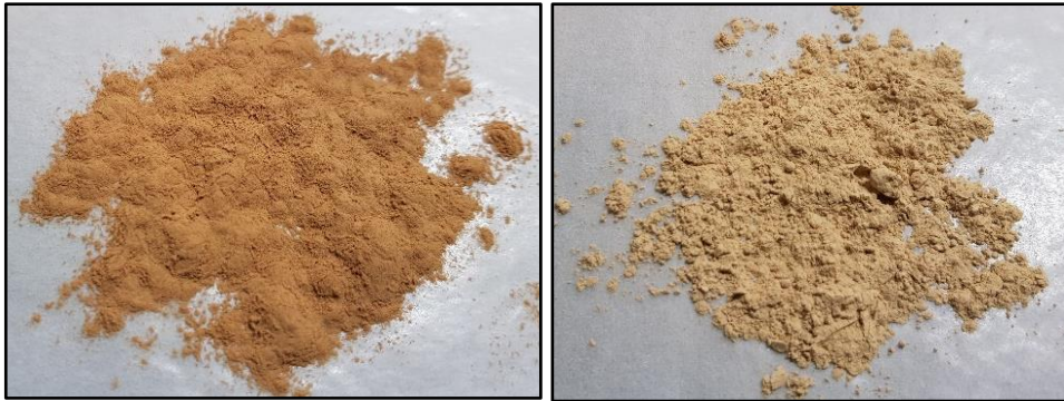
Figure 5.1: Dust found at Jordan I power plant in Jordan March 16 th , 2019. The right picture visualizes the panel dust and the left image shows the sieved ground dust.
