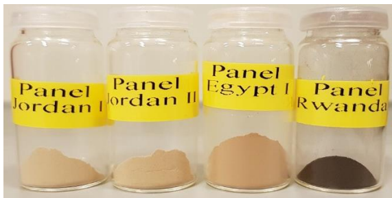
Figure 4.17: Prepared samples of panel dust from the four sites. Note the adhesion of the panel dust from Rwanda I onto the glass surface.
