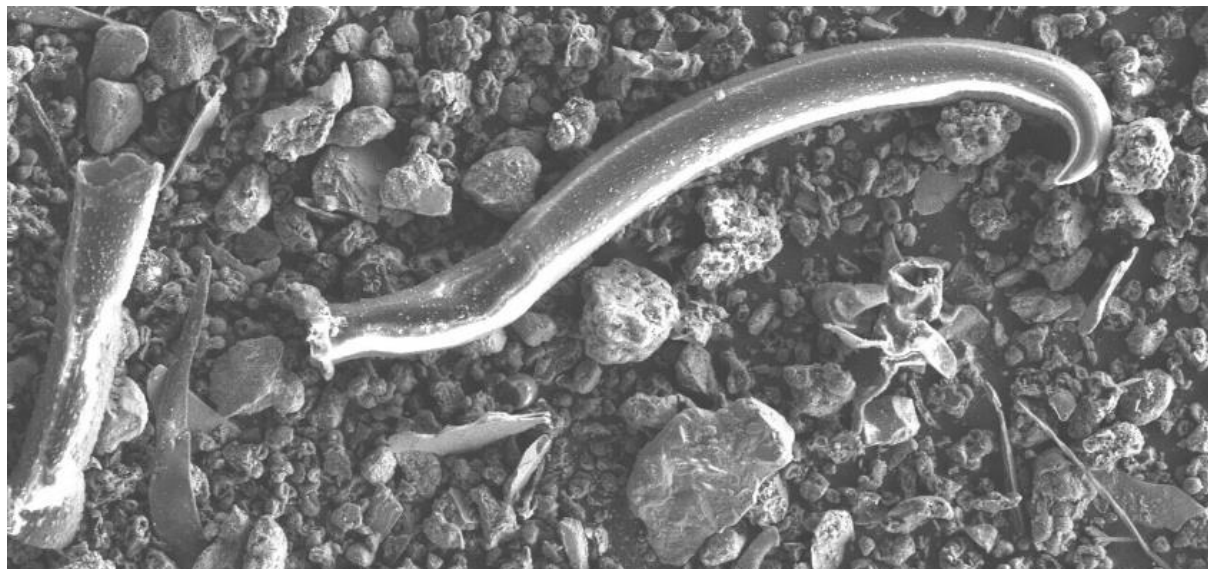
Figure 5.32: The collected dust with cloths from Rwanda I contaminated the samples significantly. The two large particles visible in the picture are clearly from a cloth and has a high value of carbon compared to the identified dust particles. Also, other particles with irregular shape is believed to be pieces of cotton.
