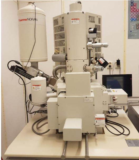
Figure 4.19: Hitachi S-4800 Scanning Electron Microscope (SEM) at Institute for Energy Technique, serial number: 9114-04.
