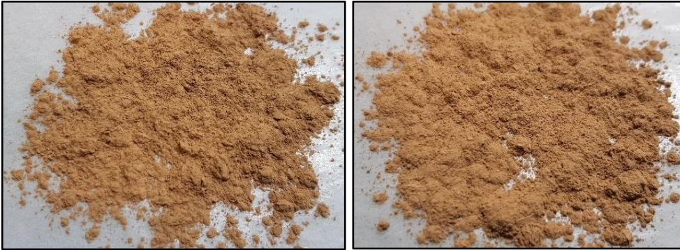
Figure 5.9: Dust collected at Egypt I on March 19 th – 20 th , 2019. The left picture shows sieved ground dust (63 µm mesh size). The right picture visualizes the panel dust.
