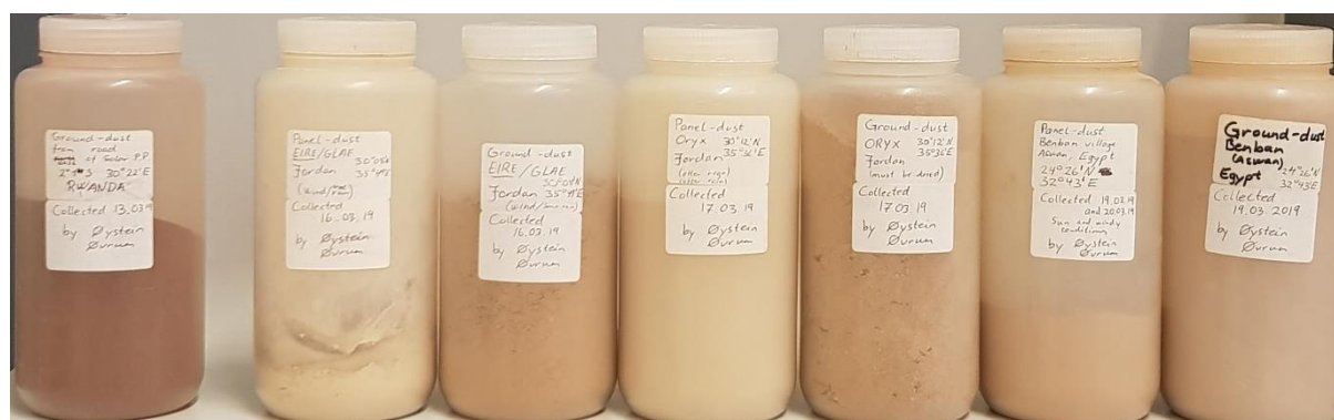
Figure 4.5: Collected dust samples from panel and ground at all locations, except panel dust from Rwanda I (insufficient amount). From left: Ground dust Rwanda I, panel dust Jordan I, ground dust Jordan I, panel dust Jordan II, ground dust Jordan II, panel dust Egypt I, ground dust Egypt I.
