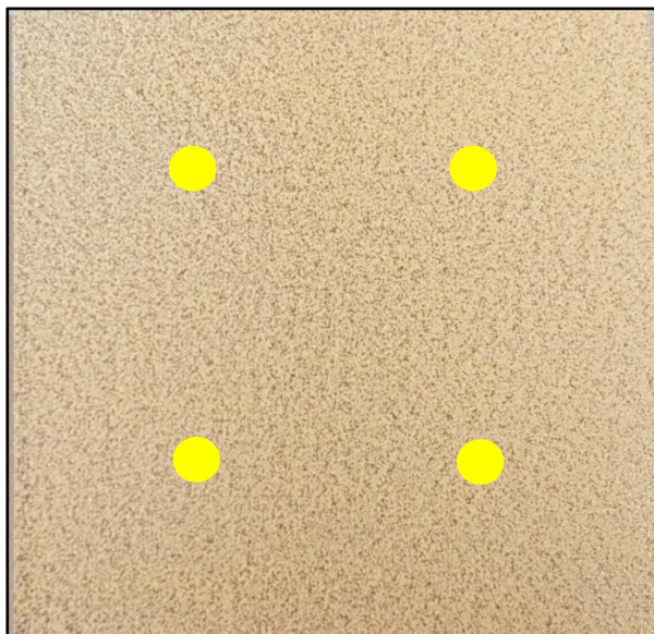
Figure 4.28: Four points (in yellow) on each sample were selected for transmission measurements with the spectrometer, in order to quantitatively assess the homogeneity of the dust layer.
