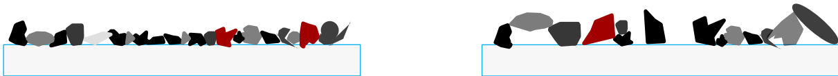
Figure 5.29: Two panels with equal density of dust, but different grain size distribution, will have dissimilar effect on the transmission of sunlight. The situation to the right clearly will transmit more sunlight than in the left situation.
