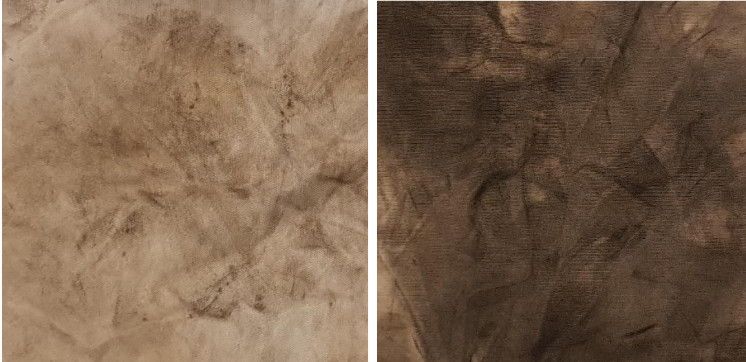
Figure C.1: Difference between dust cleaned with a cloth before (left) and after (right) the rainfall on March 14 th at Rwanda I power plant.
