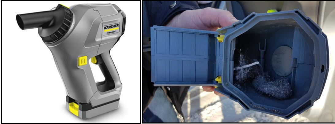
Figure 4.6: Kärcher HV 1/1 Bp Fs (left). The dust is collected in a container right after it is blown through the black cylinder, where it can be collected (right).
