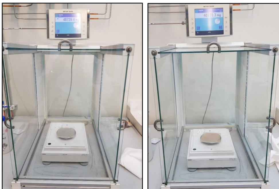
Figure 4.29: Density measurements calculated from the difference in mass weighed before (left) and after (right) dust deposition. In this particular example the mass difference is 39.9 mg, resulting in a density of ca 6.23 g/m 2 .
