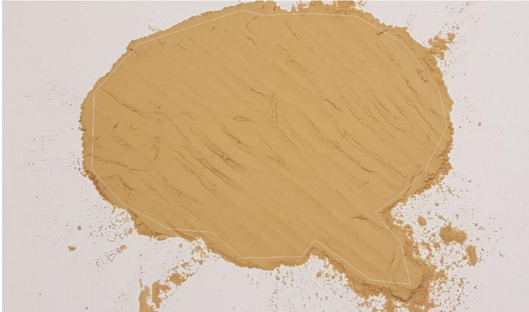
Figure 4.18: Prepared panel dust sample from Jordan II for albedo measurement by ImageJ. The selected area is marked with a thin white line.
