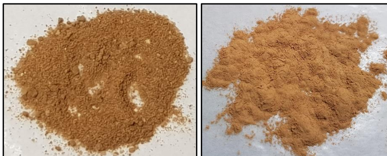
Figure F.2: Visual comparison of raw ground dust (left) and sieved ground dust (right) from Jordan I. Collected 16 th March 2019. The ground dust was sieved with 80 \mu\text{m} mesh size.
