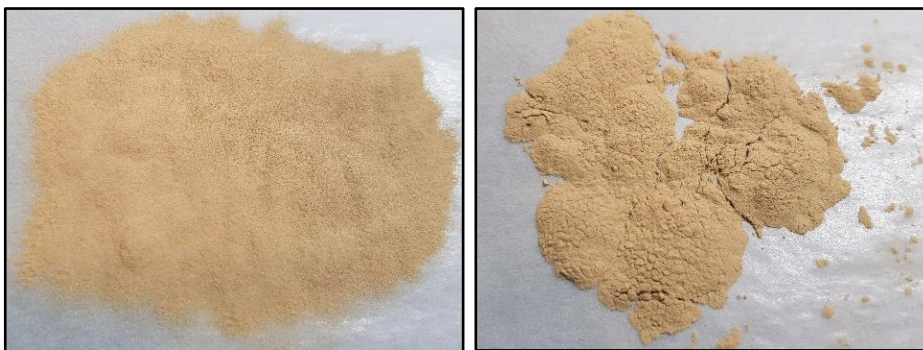
Figure 5.5: Dust collected at Jordan II on March 17 th , 2019. The left picture shows sieved ground dust from between the panel rows. The rightmost picture visualizes the panel dust.
