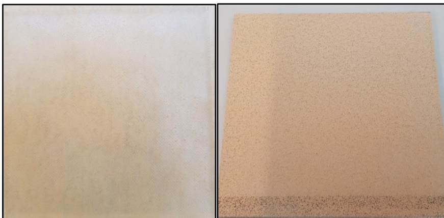
Figure 4.27: Example of non-uniform (left) and uniform (right) deposition of dust on glass plates. The validation was done qualitatively with a naked eye.
