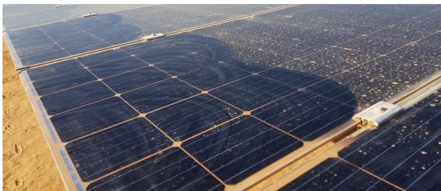
Figure 4.13: Collection of dust in Egypt I on March 19 th – 20 th . The darker part is where the panel was wiped clean with the gloves. The small dots with agglomerations of dust on the panel was a consequence of dew formations or mist that had occurred in the night.
