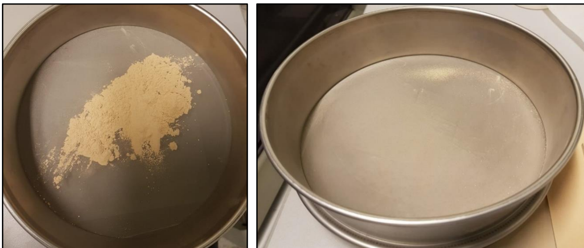
Figure 4.30: The initial amount of dust (left) and the rest after sieving (right). The picture represents panel dust from Jordan II.
