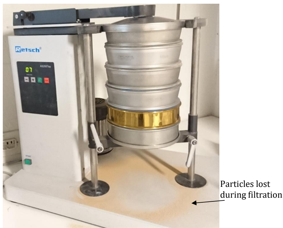
Figure 4.25: Retsch AS200 Tap sieving device was used for filtering the ground dust samples to replicate the panel dust size distribution.
