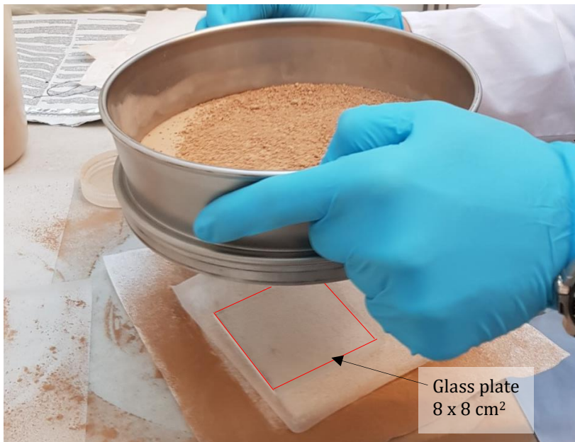
Figure 4.26: Sieving of dust for uniform deposition on 8 x 8 cm 2 glass plate. The sieve has a diameter of 20 cm and mesh size 80 µm (20 µm for cement).
