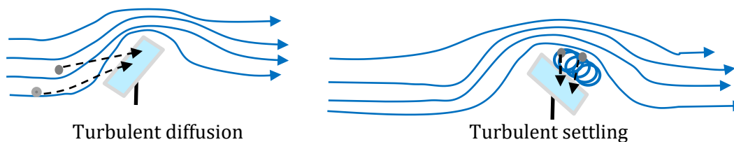
Figure 3.9: Descriptive drawing showing a photovoltaic module facing the wind (left) and a module facing the opposite direction of the wind (right). Blue lines represent streamlines of the wind, whereas black dotted lines indicate a possible pattern for a dust particle. The turbulent settling, due to gravitational forces, has the highest deposition rate among the two types depicted.
