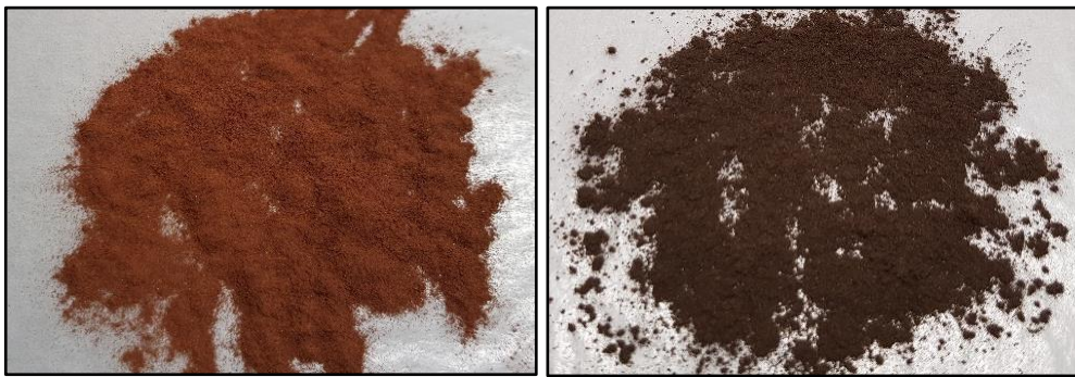
Figure 5.13: Visual comparison of dust from Rwanda I. The sieved (80 µm) ground dust (left image) was collected from a road east of the power plant. The right picture shows the panel dust.
