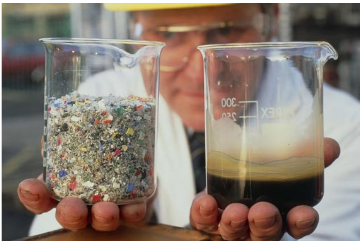
FIGURE 2: PICTURE SHOWING PLASTIC BEFORE AND AFTER BEING PYROLYZED INTO BIO-OIL [18]
