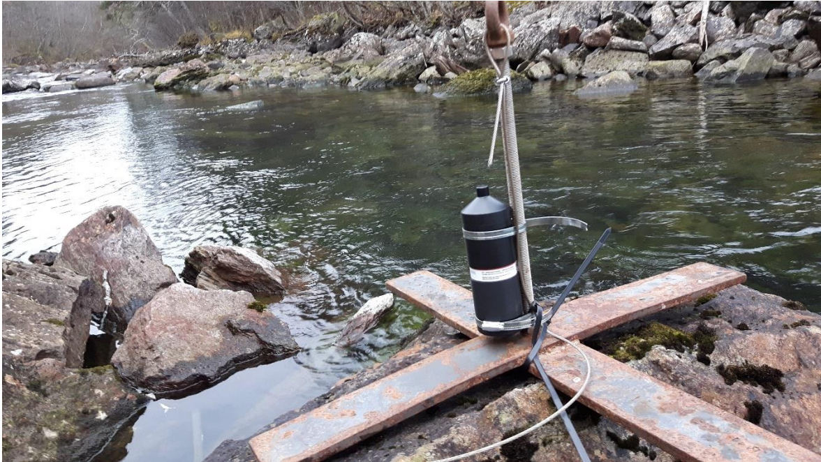
Figure 2.7: Picture of how the TBR receiver deployed in the rivers were mounted
