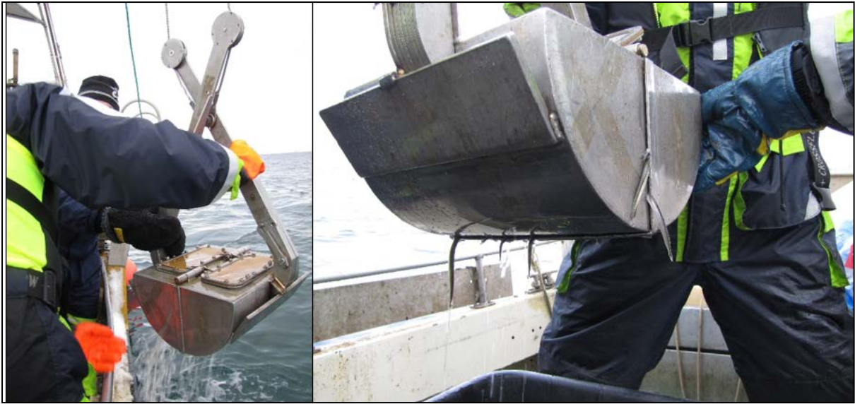
Figure 3. Sampling was conducted using a Van Veen grab deployed with a wire-winch from the boat at between 3 and 5 times at each sapling station (5 times in the M-zones).
