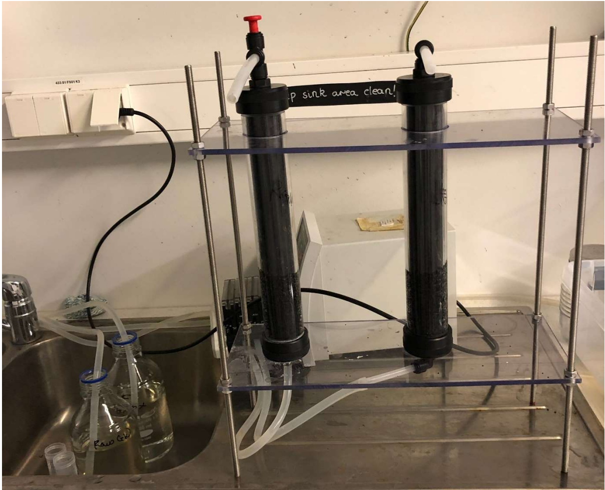
Figure 15: laboratory setup of Granular Activated Carbon filtration
