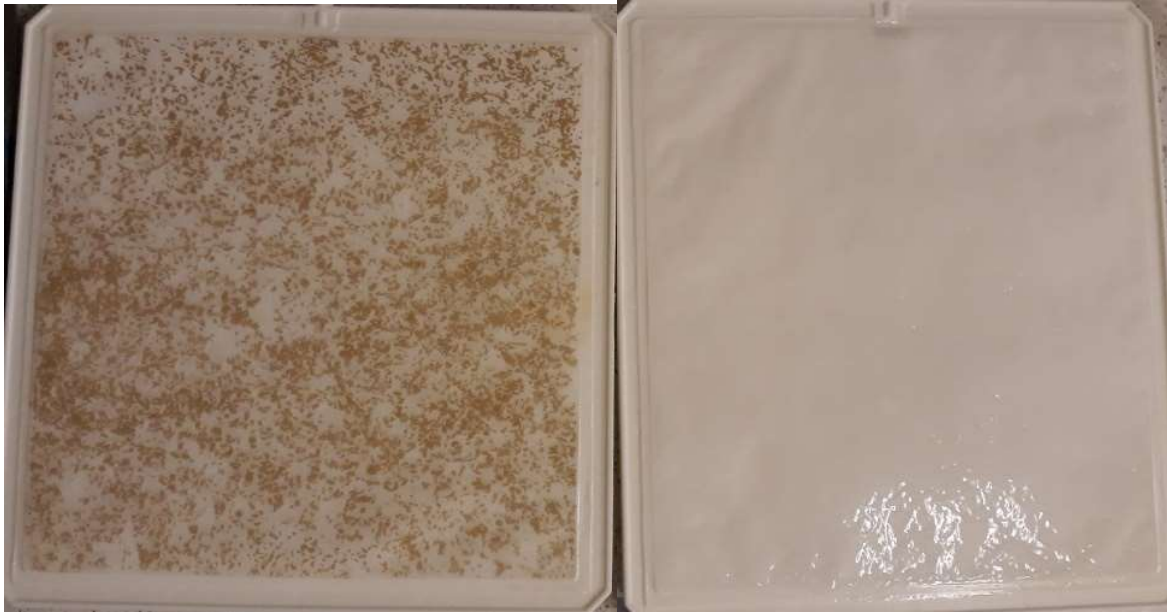
Figure 26: nano filter used before GAC (left) and nano filter used after GAC (right)
