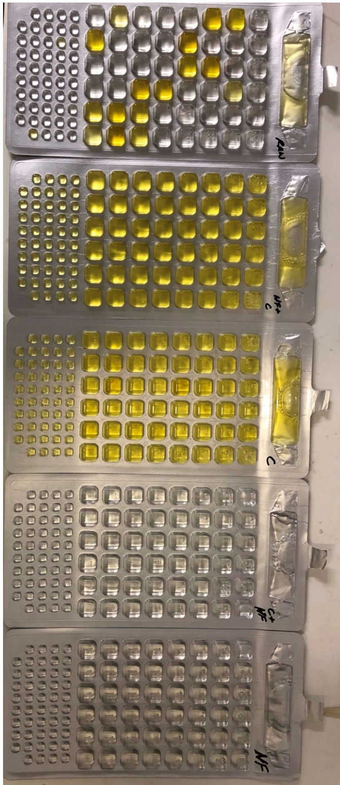
figure B- 1: samples of raw treated greywater, nano+GAC filtrate, GAC filtrate, GAC+nano filtrate and nano filtrate in Colilert 18/Quanti-trays 2000 after keeping them at 32°C for 18 hours
