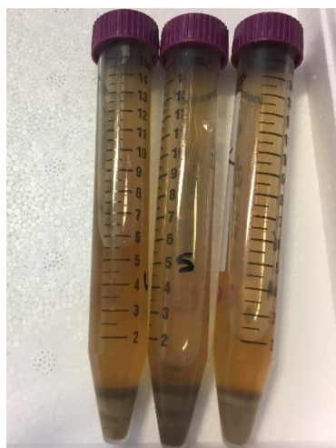
Figure 20 Digestate samples with precipitates settled in the bottom of the tubes. From left to right (1) sample after Experiment 2, (2) Sample after Experiment 3 and (3) Sample after Experiment 4
