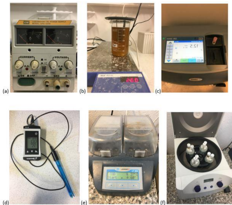
Figure 18 Equipment used in experimental work (a) DC power supply (b) magnetic stirrer (c) Hach Lange analyzer (d)pH meter (e) Hach Lange digester (f) Centrifuge apparatus
