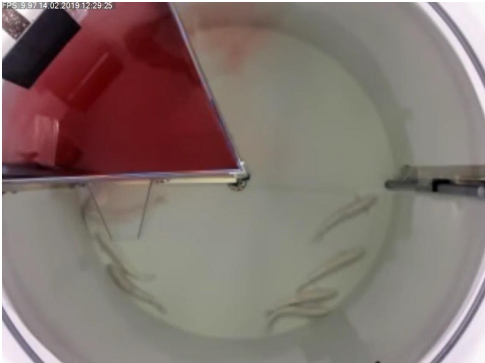
Figure 5: Food-color test. Food-color were pumped into the inlet pipe in the feeding area to demonstrate the flow through the hatches. The lack of color streaming out of hatch one, indicates a low flow through the hatch.
