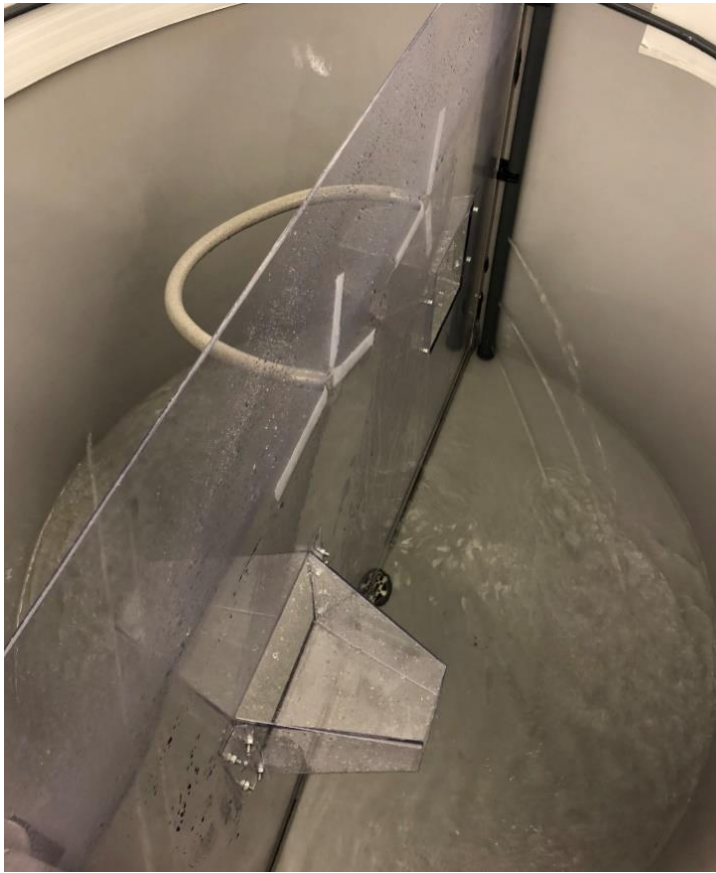
Figure 1: Tank set-up with the plexiglass wall dividing the tank into two sides, with attached hatches to facilitate one-way trafficking of fish. The hatch-design used in all experiments, with the exit opening varying between 10cm*10cm and 7cm*7cm testing different sizes. The inlet pipes with the vertically holes directing the water flow along the walls of the tank.
