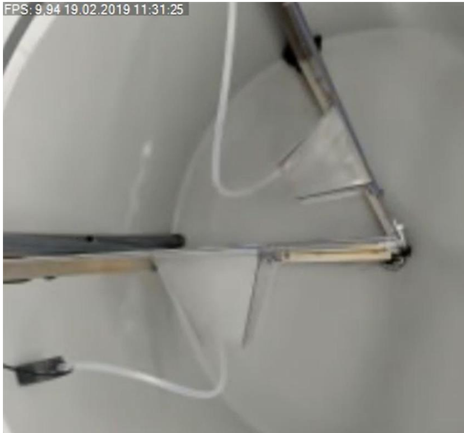
Figure 6: Feeding area with pumps attached to the tank wall, with tubes leading to the hatches exit pumping water through the hatches, increasing the flow.
