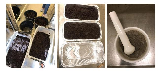
Figure 6a-c): Soil sample preparation, a) initial homogenisation of total soil sample, b) homogenisation of soil subsample, and c) crushing of soil sample.
