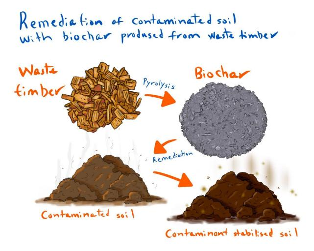
Figure 2: Concept sketch; stabilisation of contaminated soil through remediation with biochar produced from waste timber.
