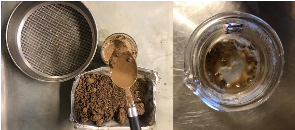
Figure 4.4 (left): The soil aggregates (tray) and muddy texture (spoon). Large particles above 2 mm are presented in the sieve (upper left), Figure 4.4 (right): The reaction between HCl and \text{CaCO}_3 in the soil sample
