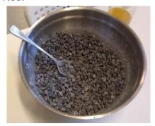
Figure 7.13: Mixing of water, calcium carbonate and LECA balls
