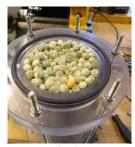
Figure 7.6: The reactor packed with peas
