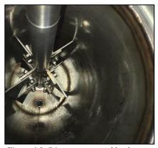
Figure 4.3: Stirrer constructed by the workshop at NMBU.
