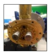
Figure 4.20: The inside mechanics of the gear pump
