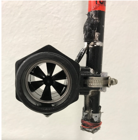
Figure 36 Self-made modifications to the water velocity meter
