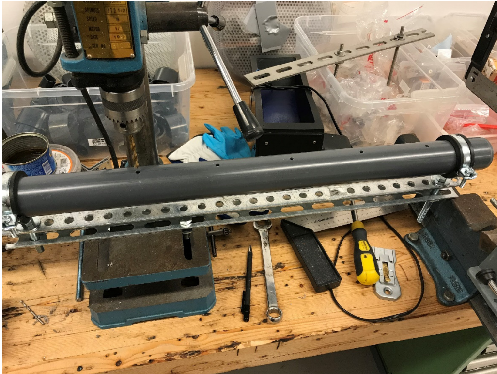
Figure 34 fabrication fixture for drilling of nozzle holes
