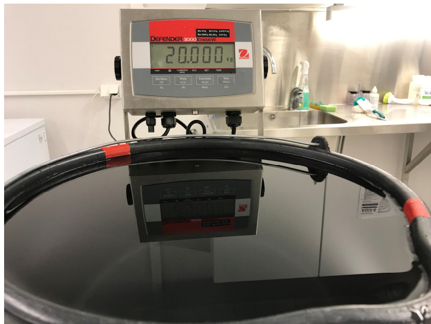
Figure 39 Bucket calibration for manual flow measurements
