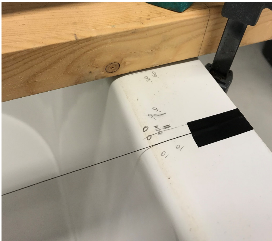
Figure 88 Centerline ( z=0 mm), beam positioning ( z=60 mm) and cord-line markings ( z=10 mm)
