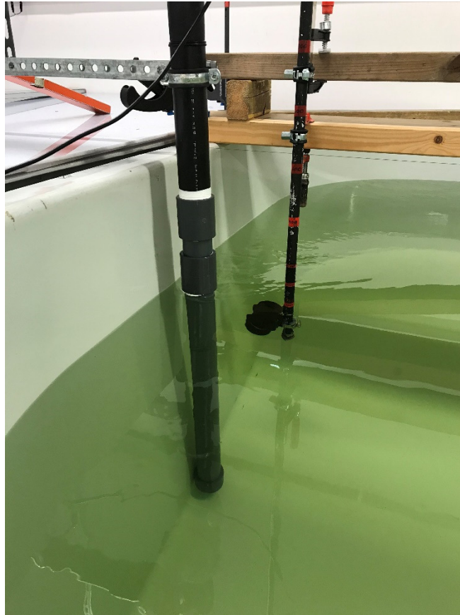
Figure 35 Inlet pipe positioned adjacent to the wall
