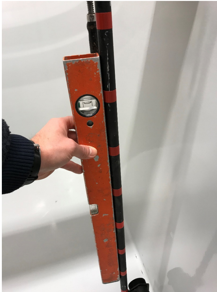
Figure 91 Demonstration of verticality assurance method
