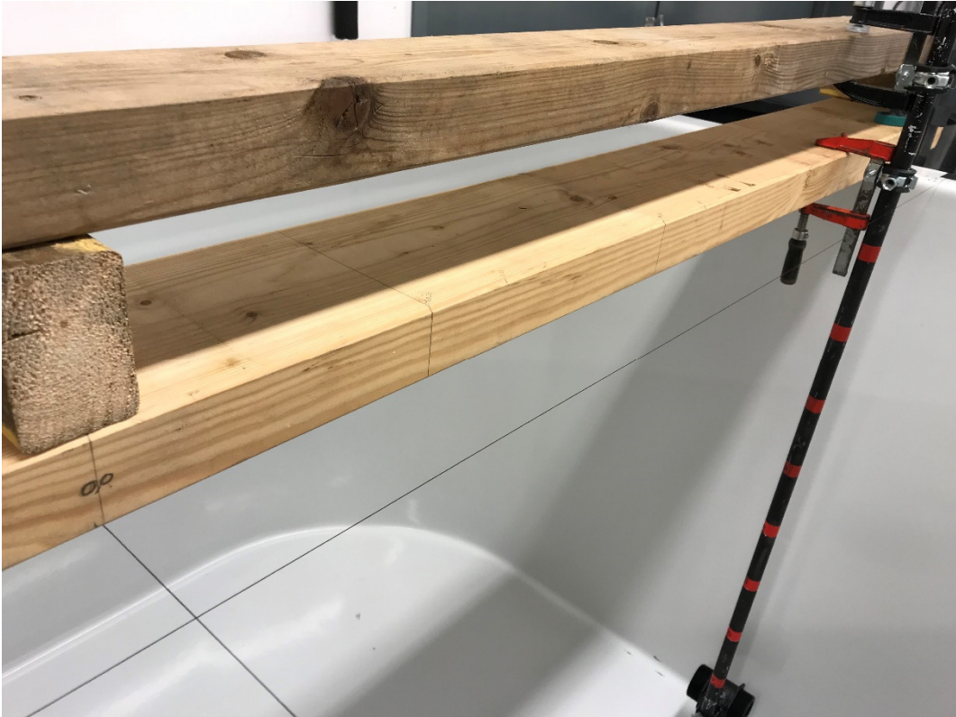
Figure 87 Sampling markings on support beam
