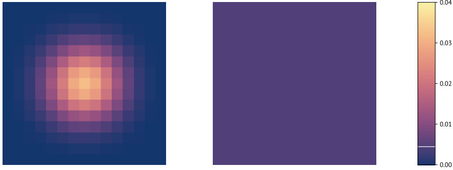
Figure 2.6: Demonstration of how the effective receptive field is different from the theoretic receptive field. The left figure shows the relative influence of each pixel on the output of a composition of seven convolutions, each of size 3. The right figure shows the relative influence of each pixel on the output for a single convolution of size 15. The white line in the colour bar shows the influence of each pixel on the output of a single convolution of size 15.
