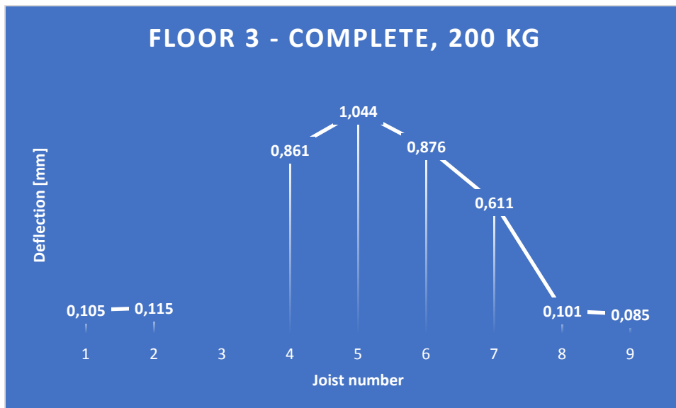
Figure 4.11 - Joist deflections from concentrated load for floor 3, bare and complete
