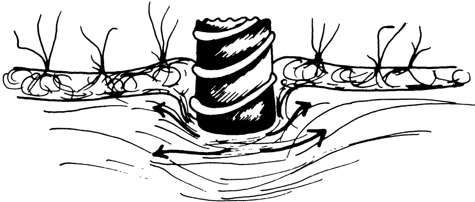
Fig. 9. Schematic presentation of the effect of a grass root mat on a peat soil.
