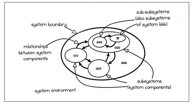
*Figure 3 – A model of a systems map showing components, subsystems, boundaries and the environment (Armstrong 2011 p137).*
