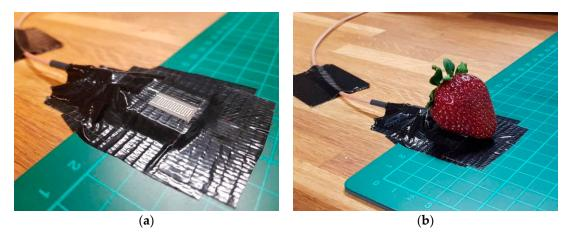
**Figure 3.** (a) 8-pair IDE sensor, with only sensitive element exposed and (b) example with fruit in place for measurement.
