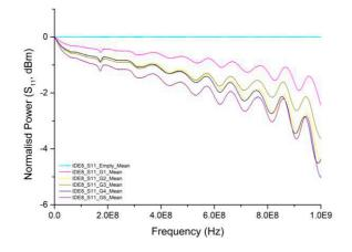
**Figure 4.** Spectral data between 9 kHz and 1 GHz; observation highlights a clear separation between the spectral data between 200 and 600 MHz.
