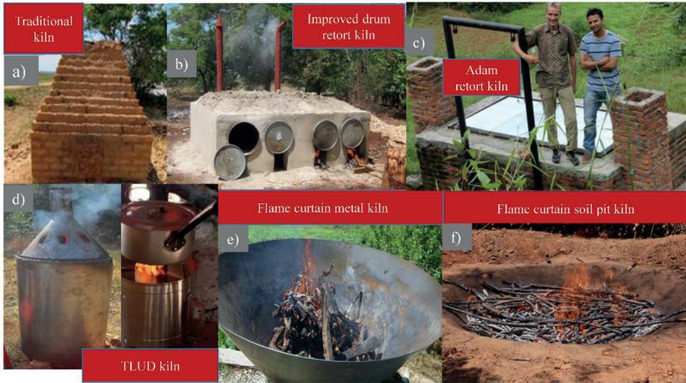
**Fig.4.** Biochar production technology; non-retort (*Fig a*) and retort kiln (*Fig b*) (Sparrevik et al., 2015); adam retort kiln (*Fig c*) (Adam, 2009); TLUD kiln (*Fig d*) and flame curtain kiln (metal kiln (*Fig e*) and soil pit kiln (*Fig f*)) (Schmidt and Taylor, 2014).
