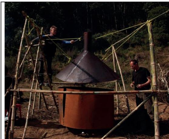
Measurement of the gas emissions using a chimney to channel the escaping gases so that they could be measured simultaneously.
