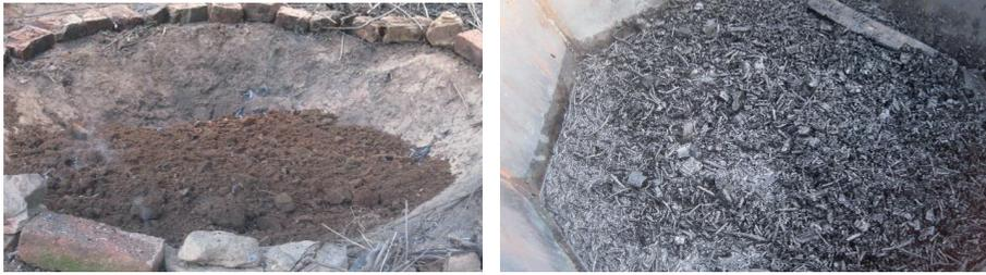
**Image 6:** Snuffing with soil (left) and water (right)
