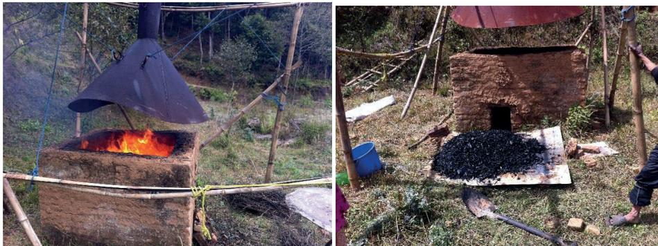
**Image 2:** Traditional brick kiln operation (left) and biochar harvested (right). Sizes : Inner wall; 1m x 1m x 1m and Outer wall; 1.4m x 1.4m x 1.4m.
