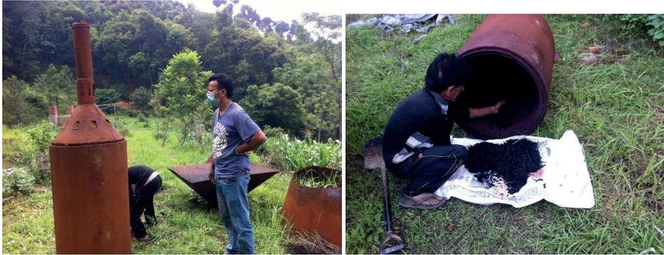
**Image 3:** TLUD operation (left) and biochar harvested (right). Sizes: 0.65 m diameter, 1.05m height and 2.2m circumference.
