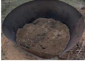
Snuffing of soil pit kiln with soil, pressed with feet and shovel to make it air-tight.
