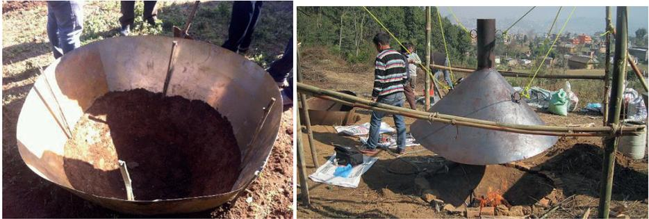
**Image 4:** Steel shielded soil pit (left), Sizes: diameter (top: 1.02m, middle: 0.8m and bottom: 0.47m), height: 1.55m, and Conical soil pit (right), Sizes: diameter (top: 0.8m, bottom: 0.47m), height (0.8m).
