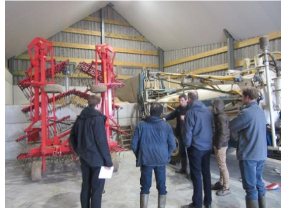
FIG 16: FARMERS DISCUSSING BETWEEN THE TINE WEEDER (LEFT) AND VINASSE SPREADER (RIGHT). 28/03/2018 IMAGE BY RAPHAEL BOUTSEN.
