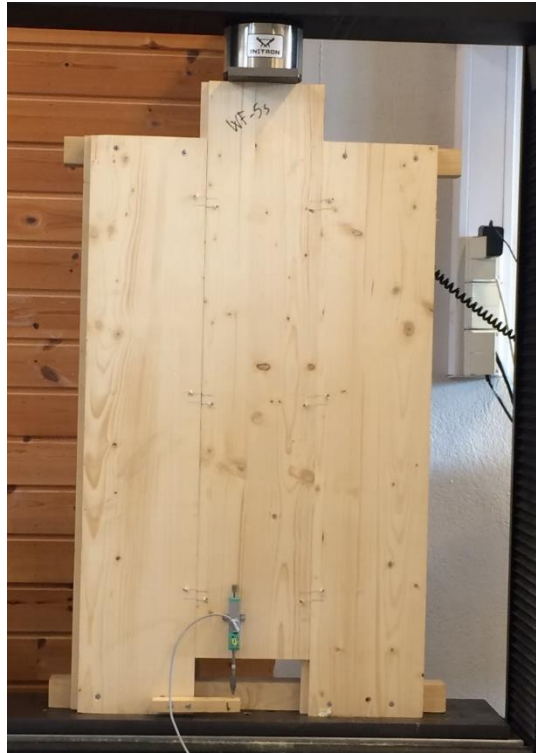
Figure 3-22: Study 3 specimen with fasteners ready for testing in the Instron machine.
