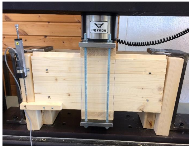
Figure 3-16: Study 1.2 cyclic load test specimen during testing in the Instron machine.
