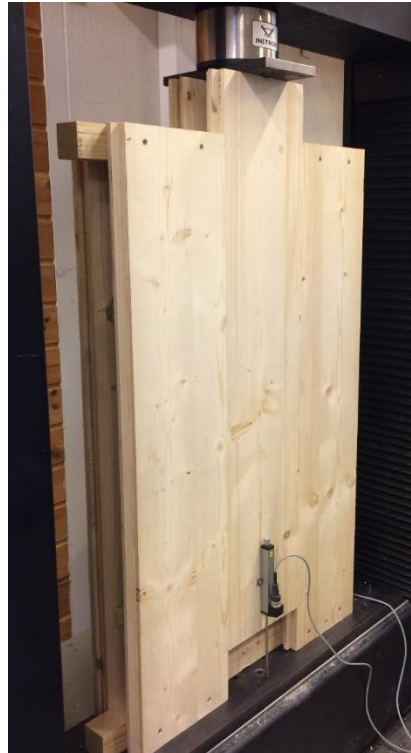
Figure 3-23: : Study 3 specimen without fasteners ready for testing in the Instron machine.
