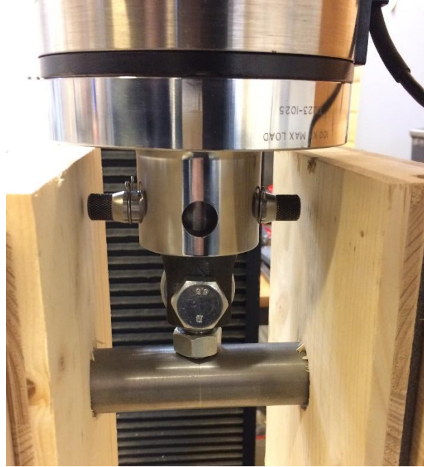
Figure 3-19: Study 2 Instron cell tube-connection set-up.
