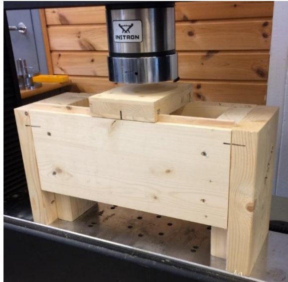
Figure 3-14: Study 1.1 monotonic load test specimen ready for testing in the Instron machine.
