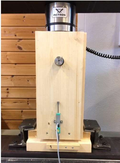
Figure 3-18: Study 2 specimen ready for testing in the Instron machine.
