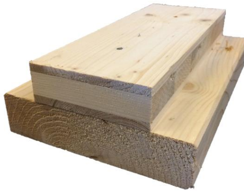
Figure 3-7: Bottom sill connected to a middle sill of SWP material.
