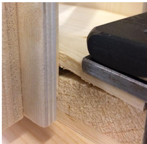
Figure 5-1: Photo of HSS7s during study 2 testing, showing the separation between lamellas in SWP middle sill.
