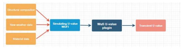
Figure 3- Figure describing the methodical approach of calculating U-value with Wufi.
