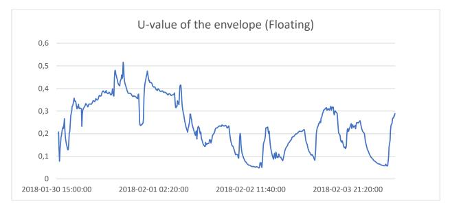
Figure 37 - Graph showing the varying U-vale calculated from the measured heat flux and delta T.
