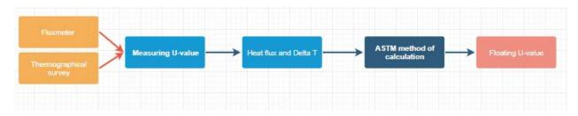
Figure 4- Figure describing the methodical approach to determining U-value through measurements.
