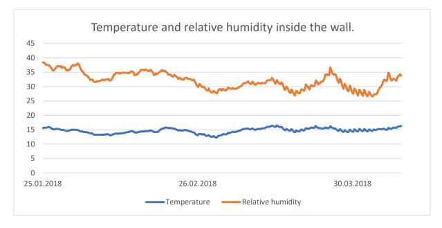
Temp and RH measurements from inside the envelope 25.01.18 to 30.03.18 is seen in Figure 41:
