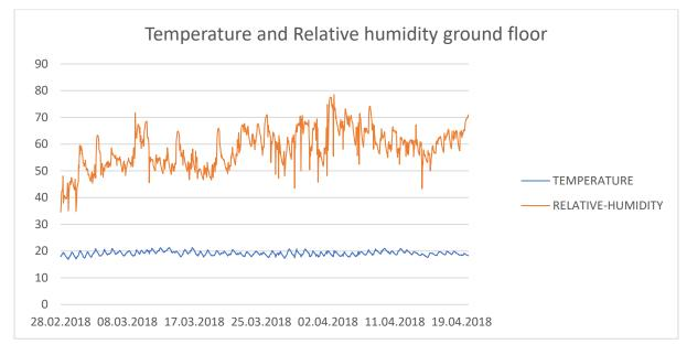
Figure 40- Temperature and humidity measurements, ground floor apartment.
