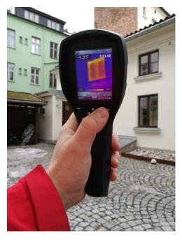
Figure 29- Using the FLIR I3 thermal imaging camera.
