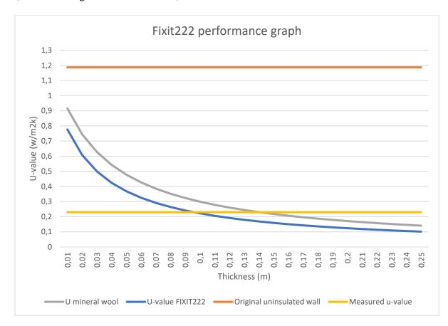
Figure 44 - Graph depicting U-values of original structure, measured new value and u-value of Fixit and mineral wool in relation to thickness applied.
