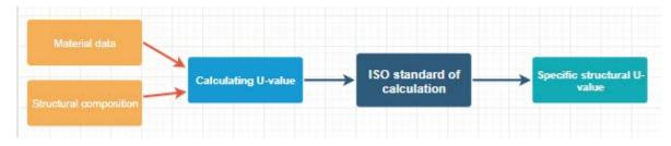
Figure 2- The methodical approach used to calculate U-vale, according to ISO standard 6946:2014.
