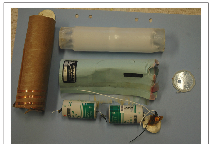
FIGURE 1 | Components of a Telonics IMP/400/L intraperitoneal VHF implant (length 15.2 cm, diameter 3.3 cm, weight 170 g). The lithium batteries, transmitter, and antenna (central bottom) were enclosed in a thick paper tube (left), wrapped in thin paper (central middle) labeled with the company’s name and address and the serial number of the device. These parts were contained within a plastic shell cylinder (central top) with both ends closed with glued-on end caps (right). The plastic shell cylinder was coated with a 2.1 mm thick wax of unknown composition.
