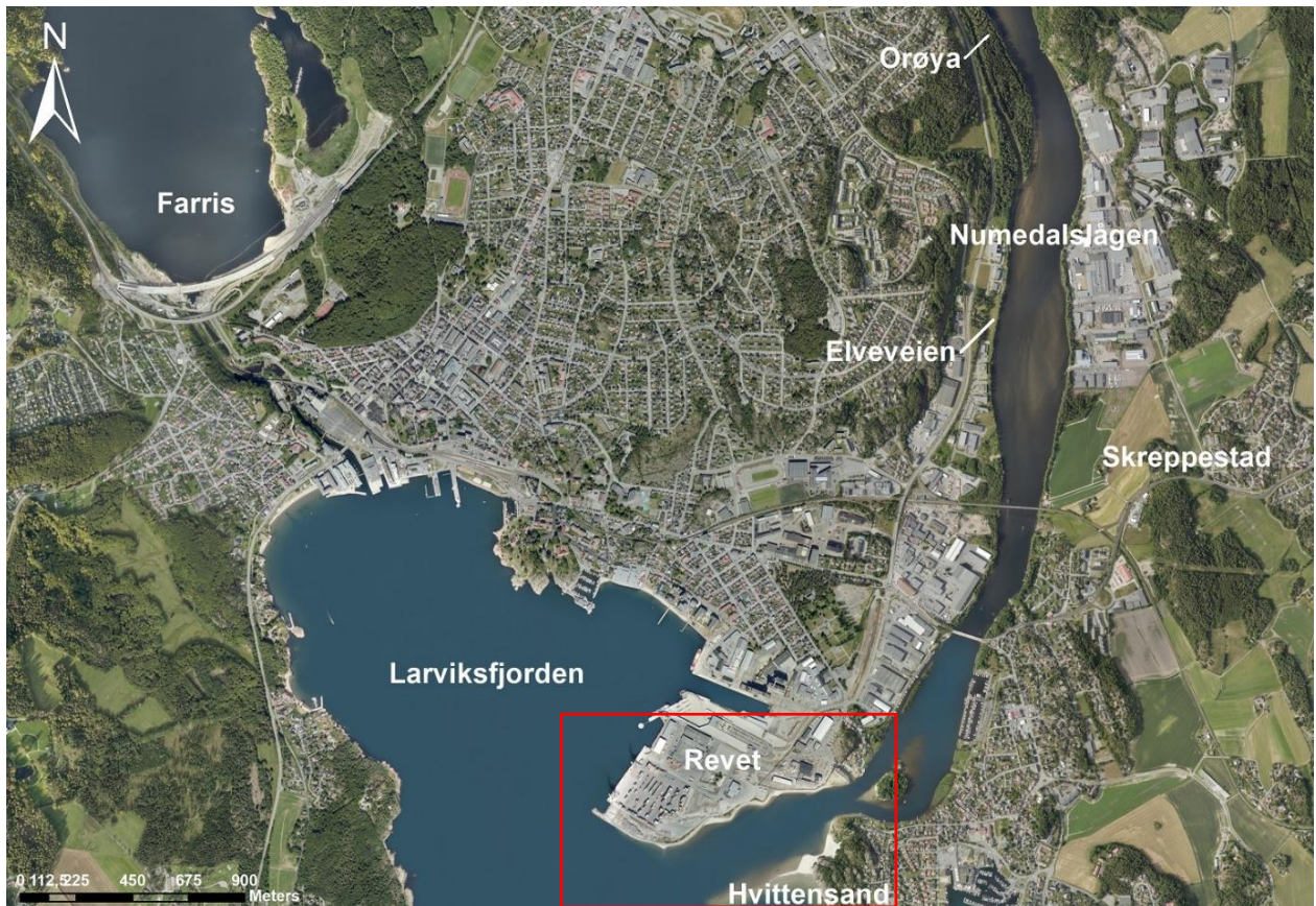
Figure 5: Aerial map of Larvik. The river Numedalslågen flows from the N and deposit sandy sediments in the investigation area (in the red square) (From Kartverkets WMS (GeoNorge, n.d)).
