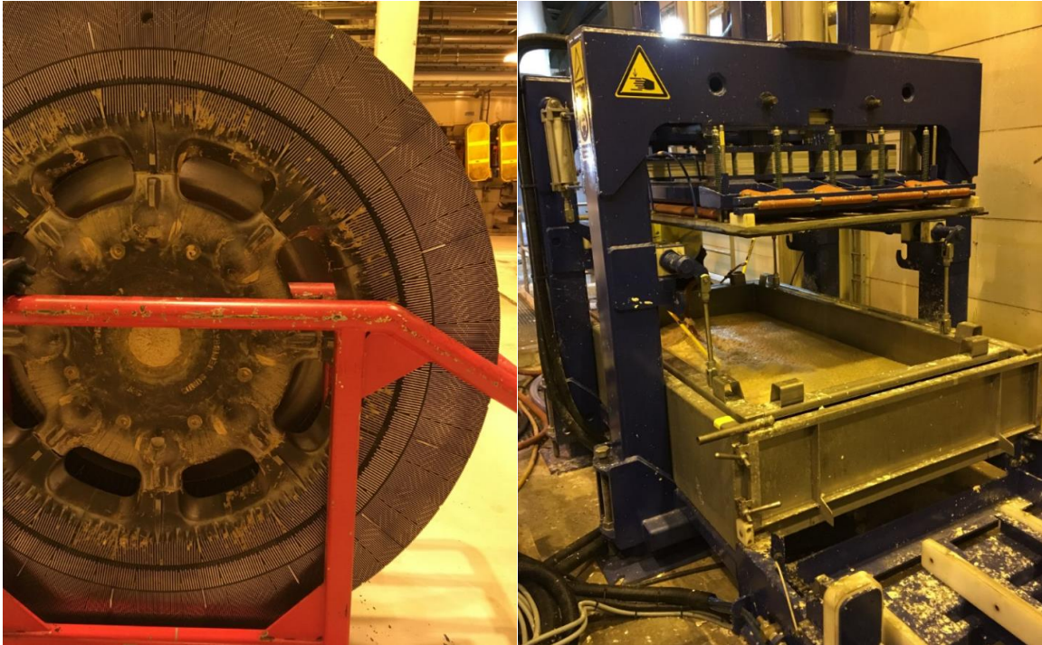
Figure 1: Refining disk used for grounding fibres and press.
