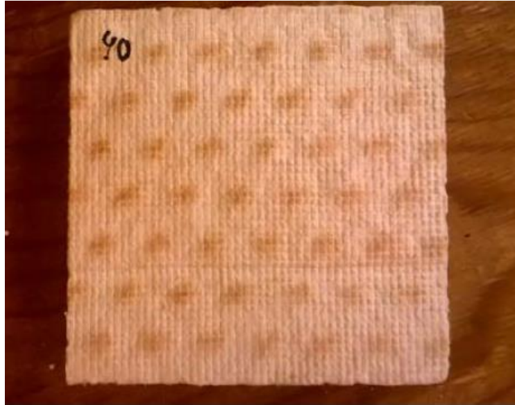
Figure 12: Sample example used in cone calorimeter. (Photo taken by Erik Larnøy, NIBIO, Ås)
