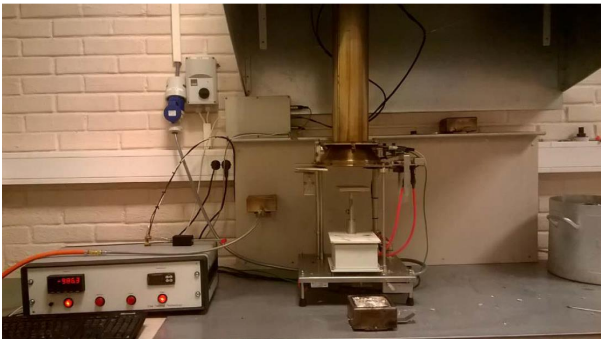
Figure 13: Setup for cone calorimeter fire testing (Photo taken by Erik Larnøy, NIBIO, Ås)
