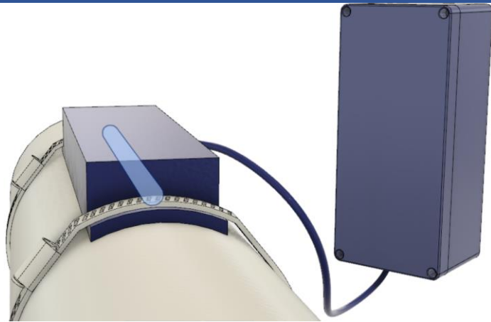
Figure 29: Small curved base enclosure, transducer highlighted in light blue.
