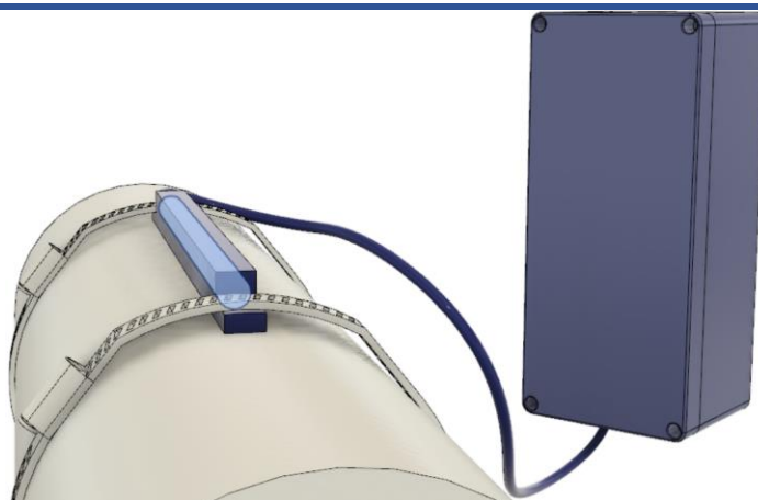
Figure 31: Minimalistic flat base enclosure, transducer highlighted in light blue.
