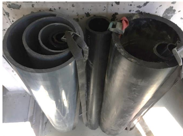
Figure 22: Meter-length pipe samples of PE and PVC pipes used at Kroksjøen Waterworks.
