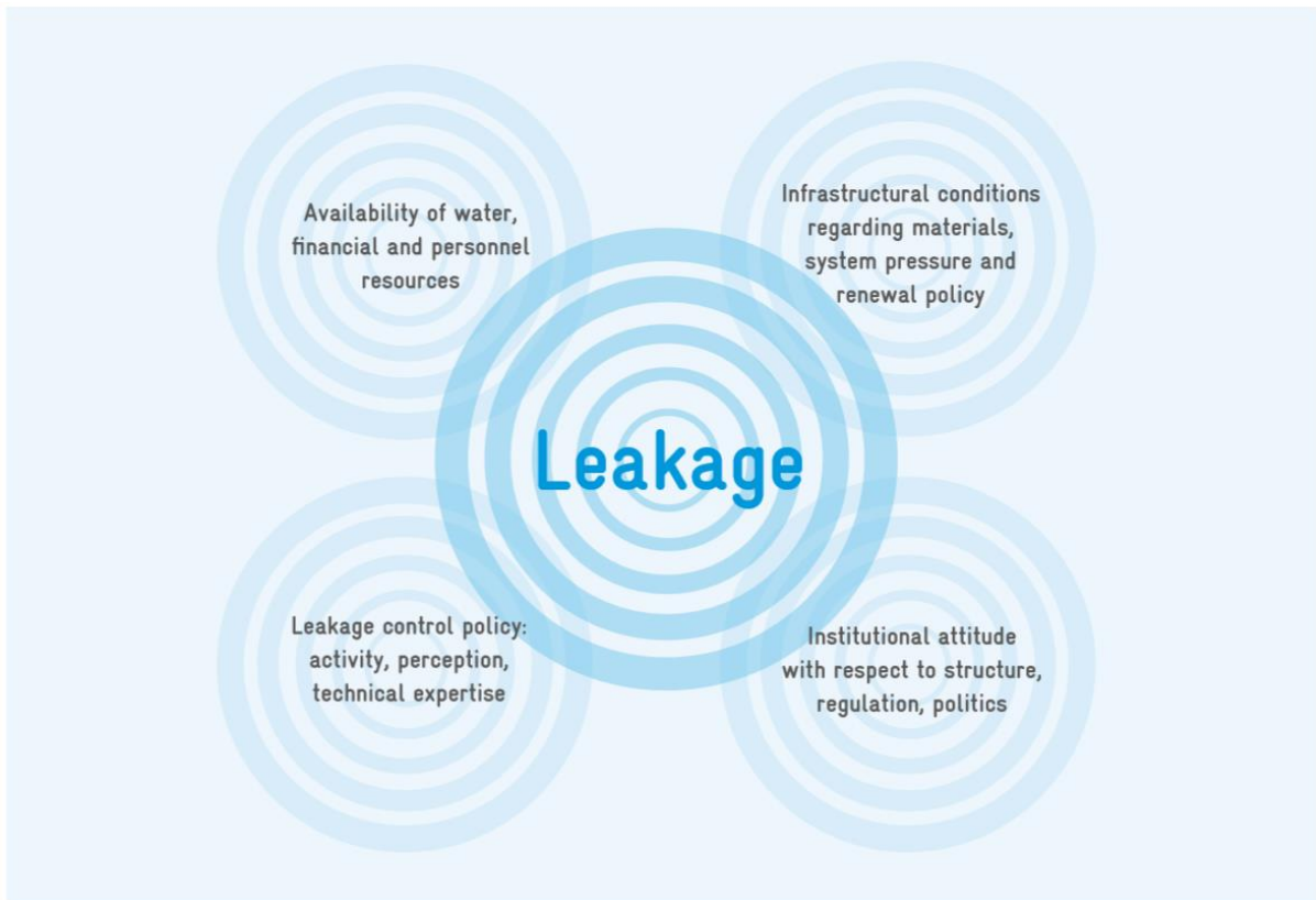
Figure 10: Key factors influencing leakage in a water utilities network. Efficient leakage management requires a good understanding of all factors [24].
