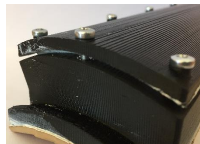
Figure 47: Gap between lid and enclosure body.
