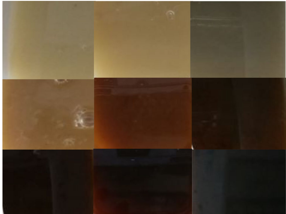
Fig. 2 The color change of steam exploded potato, using various steam explosion condition. The boxes on the top represent the potato samples with steam explosion at the lowest temperature (135 °C), the boxes in the middle are samples from medium temperature treatment (180 °C), and the boxes at the bottom represent samples from the highest temperature (215 °C). From left to right on all rows, samples treated at the stated temperature for 10, 20 and 30 min, respectively
