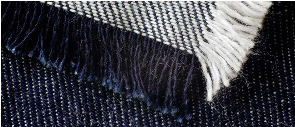
Figure 1.3.4.2. Denim fabric. Warp (blue) and weft (white) are yarn spun from cotton, pretreated with and without dyeing, respectively, and woven to denim fabric (Clariant 2012).
