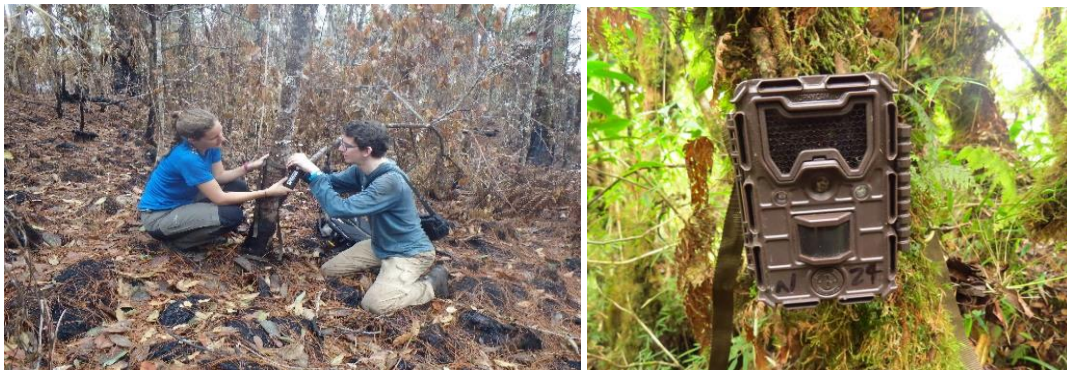
Figure 4: Positioning camera traps on trees approximately 1m above the ground
