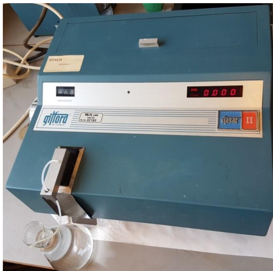
Figure 15: Gilford Stasar II spectrophotometer used to determine the P-adsorption from filtrate solution at 885 nm absorption.
