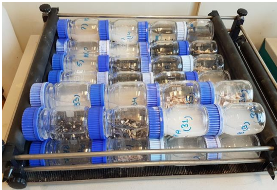
Figure 11: Showing labeled glass-bottles, filled with shell-samples and specific amount of solution (Distilled water or 330 ppm P- solution). To get mixed them properly, bottles were fixed on suspension shaker for 24 hours.
