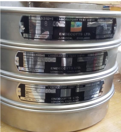
Figure 7: Demonstrating the adjustment of Sieves with respect to their pore sizes. The largest (4-8mm) is at top, medium (2-4mm) is in second number, the smallest (0-2mm) is in third number. On the bottom it is for the collection of smallest size shells material.
