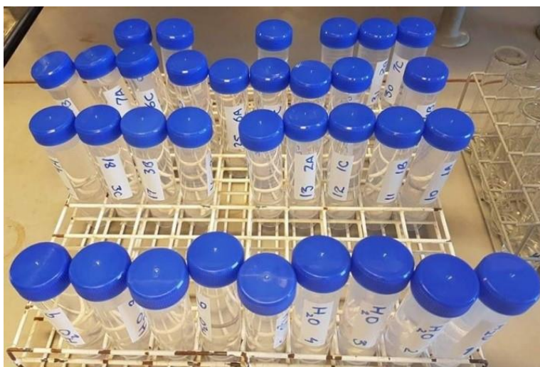
Figure 14: Showing filtrate in test-tubes after centrifuged. Tubes are placed in iron-tube stand, labeled with marker and tightened with blue cap.
