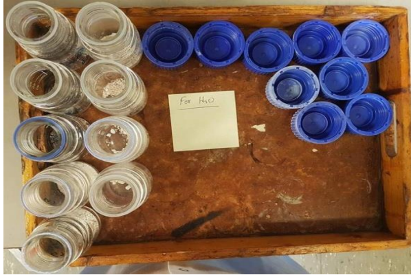
Figure 9: Glass bottles with blue screw caps having 100 ml volume. Bottles were marked from 1-9. This set-up was used as a blank analysis.
