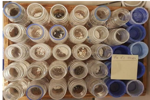
Figure 10: 27 glass bottles with blue screw caps having 100 ml volume. Bottles were marked from 10-36. This set-up was used to analyze P-adsorption of shell-samples
