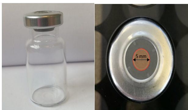
Figure 24: The red circle represents the sealed part of the vial, a circle with a diameter of 5 mm.
