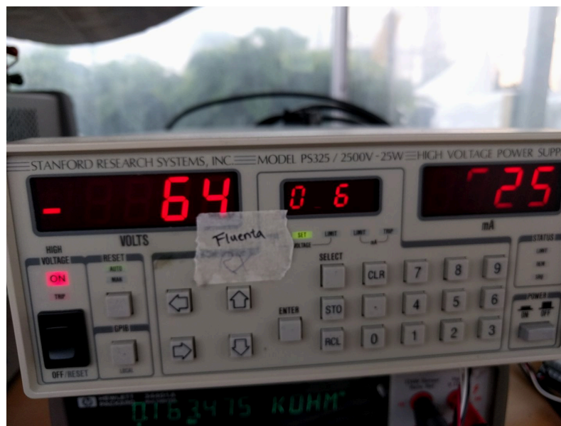
Figure 6: The SRS PS325 Power supply that supplies the CMUT sensor
