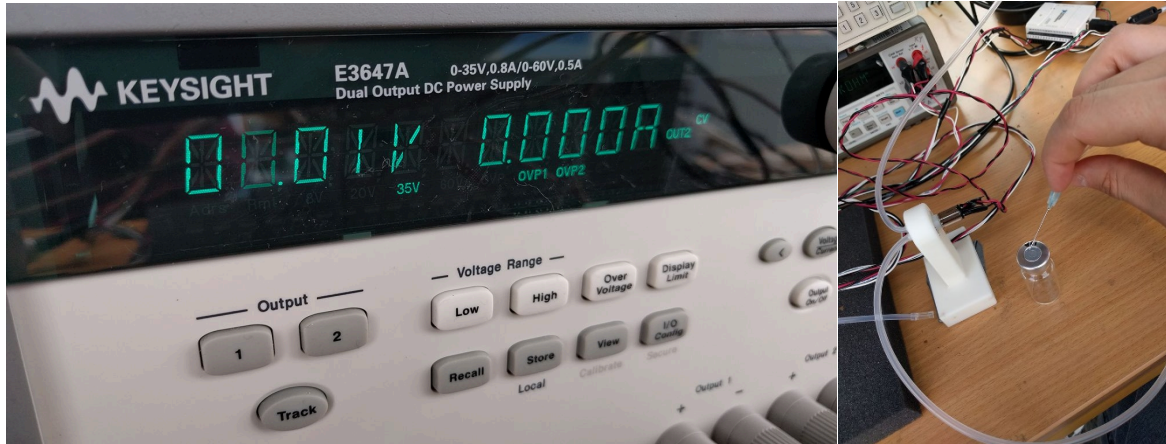
Figure 10: By using output 1 and 2 you can regulate manually the micro vacuum pumps by applying 3 Volts, the picture to the right show how to collect samples for the GC.
