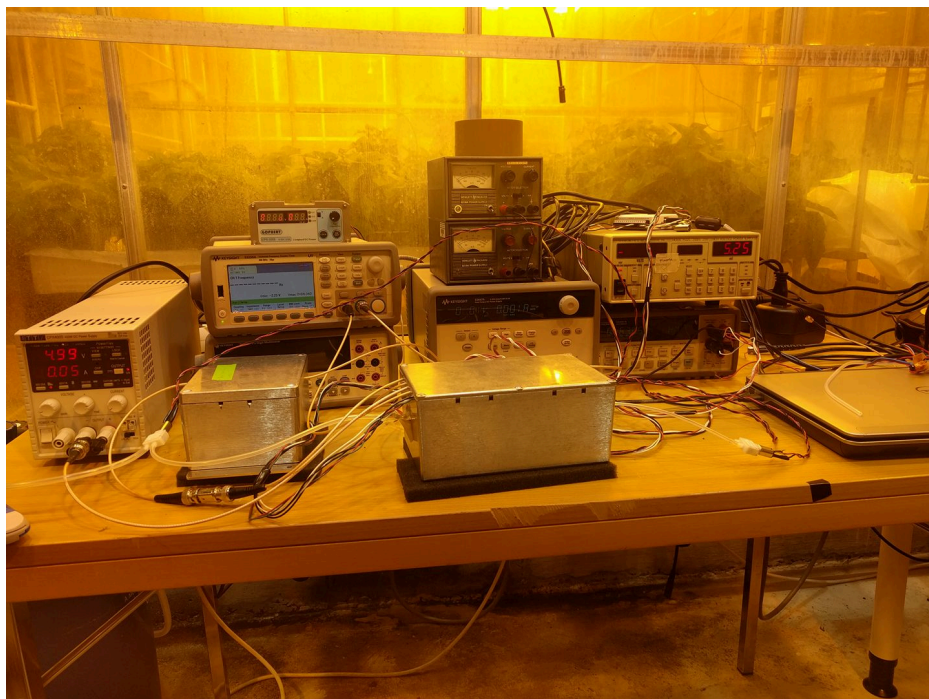
Figure 5 Overview of the electronic set up (From left to right): Power supply to pump (earth), Frequency counter, CMUT sensor and voltage regulator (aluminum boxes), power supply to pump (air), power supply to the sensor set-up, the multimeter and computer where we run the Matlab Script.
