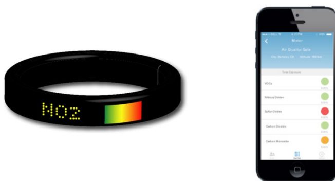
Figure 11: a) Early prototype of the CHEMISENSE bracelet. b) App that provides real-time data processing both from [57]
