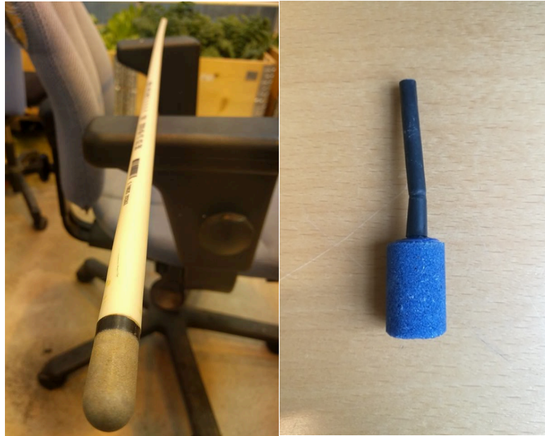
Figure 30: Different sparger types, a) ”gas measuring tube” b) bubble stone sparger
