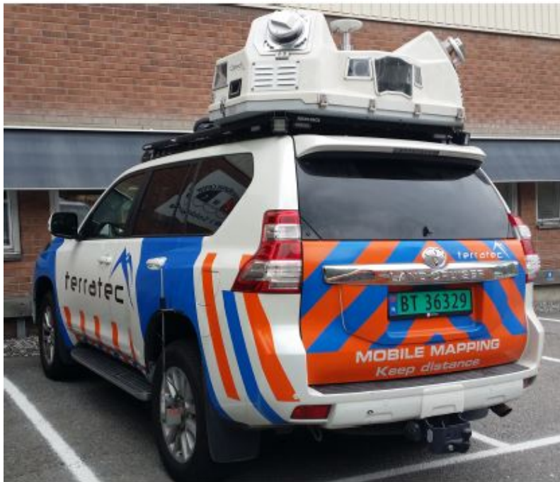
Figur 5.3.1: Optech Lynx Mobile Mapper SG1
