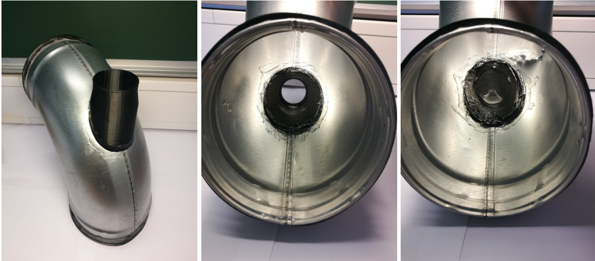
Figure 9-9: Pictures of the dispersion openings mounted to a bend, showing the sealant on the in- and outside. Further giving a view with the lid placed in the opening.
