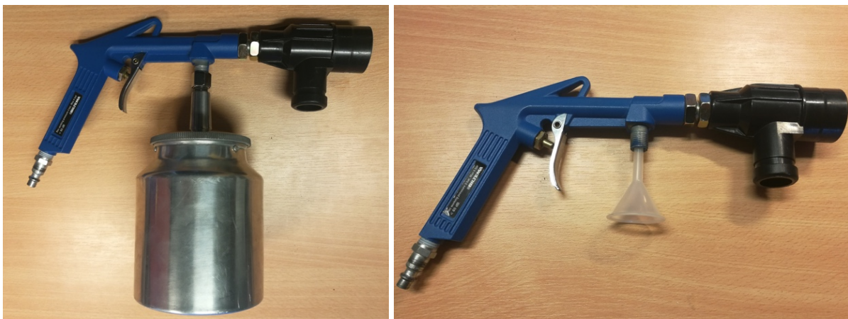
Figure 10-7: A overview of the two different methods that have been tested. Left: With the canister, Right: With the funnel.
