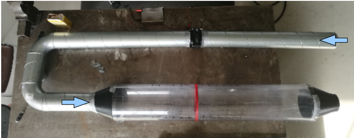
Figure 10-12: Setup used to test the rotational motion of the air, with and without the distribution device. Arrow showing the direction of the particle flow. Picture taken in-between testing.
