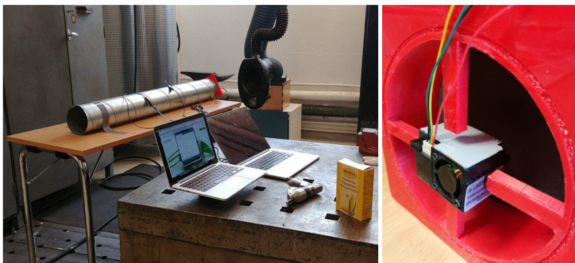
Figure 10-6: Here the experimental setup can be seen. Left: Showing two computers, only one was use at a time. Further showing the pipe which the particles enter and the suction pipe positioned behind the outlet of the pipe. Right: The sensor is fastened to the pipe using a sensor holder.
