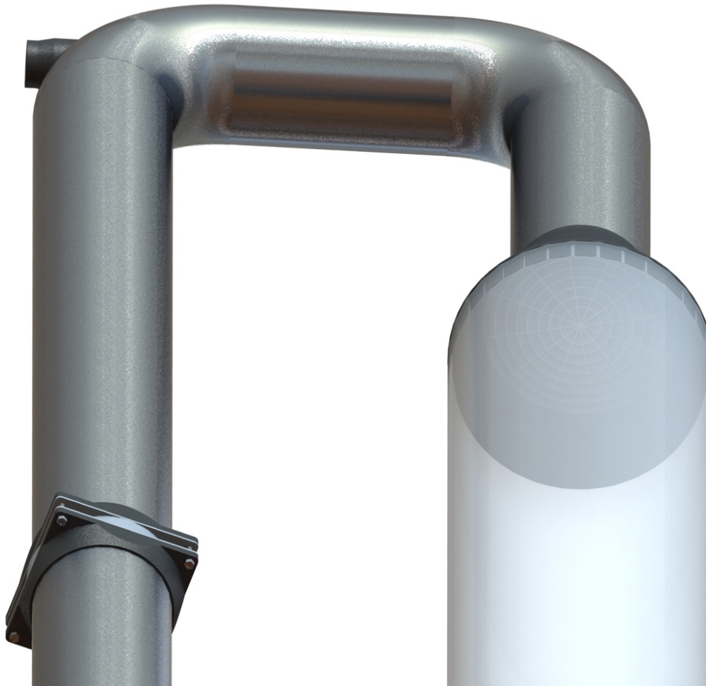
Figure 9-2: Assembly rendering from below showing the distribution device mounted in the funnel. CAD rendering made in Solidworks.
