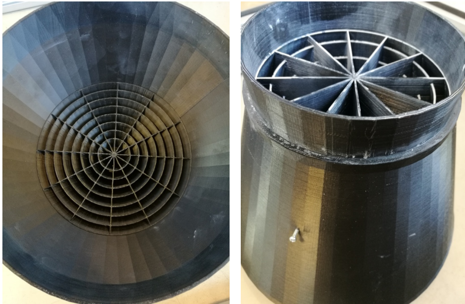
Figure 9-11: The distribution device fastened to the funnel. The white parts are powder from testing.
