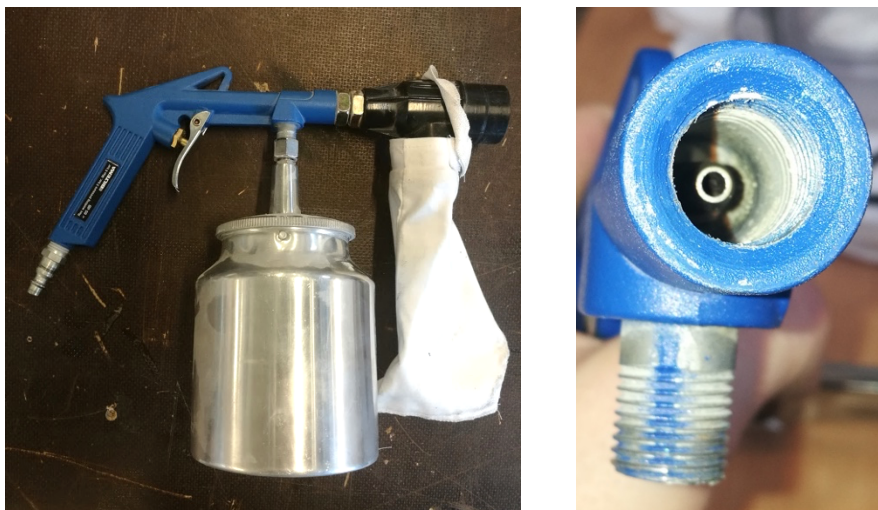
Figure 6-5: A picture of the Biltema point sandblaster and a picture of the nozzle inside the sandblaster.
