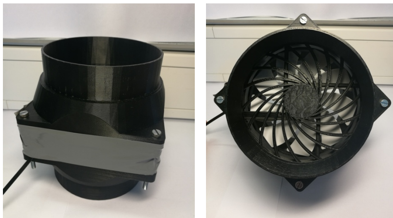
Figure 9-10: Pictures of the fan rig showing how it is fasted and seal, as well as a view through the assembly.
