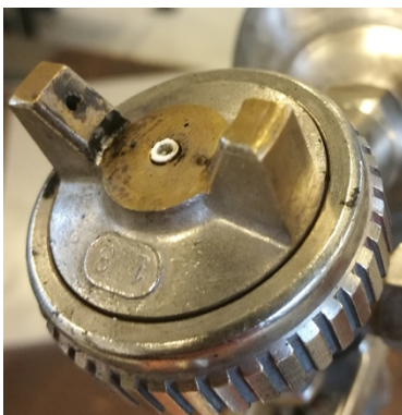
Figure 6-8: A picture of the paint gun nozzle and an illustration of how the paint atomizes a fluid or in this case particle powder. [73]
