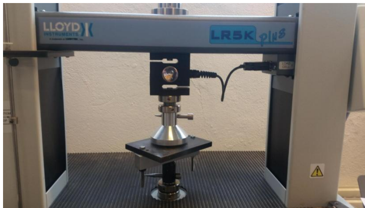
Figure 7: Hardness testing machine (Lloyd LR 5K texture analyzer)
