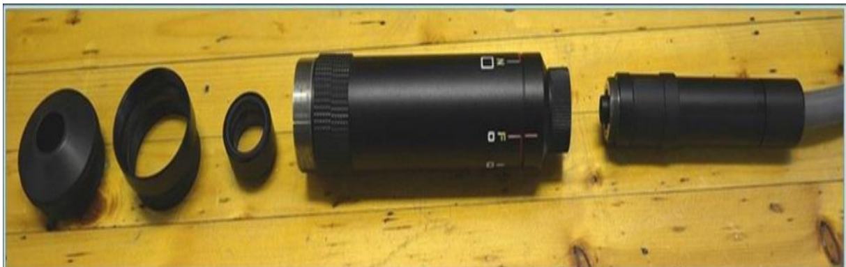
Figure 12: Setting of the video microscope: from right to left (in order of assembling): CVM video probe head from Micro Viper portable computer; Allen zoom lens, 20x – 120x basic lens; contact head adaptor; 60x-420x contact head (Misljenovic et al., 2015).
