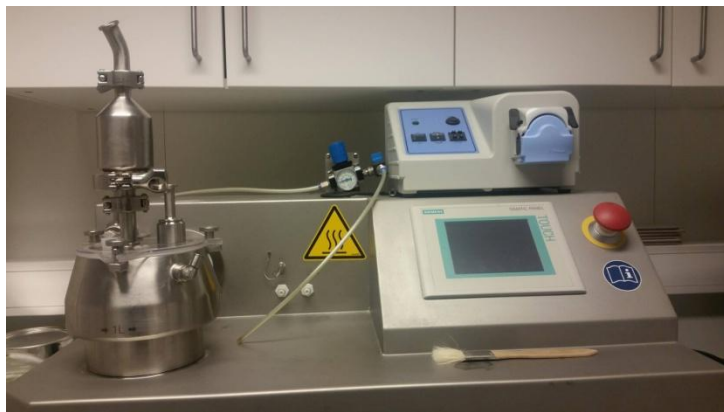
Figure 5: Lab scale mixing blender and fluid sprayer
