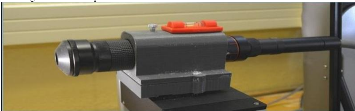
Figure 10: Assembled and fixed video microscope lens on tensiometer.
