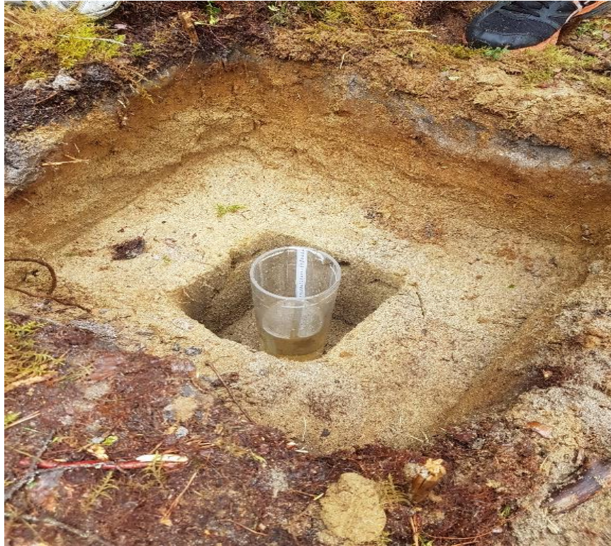
Figure 20 Modified Phillip -Dunne Infiltrometer in Field
