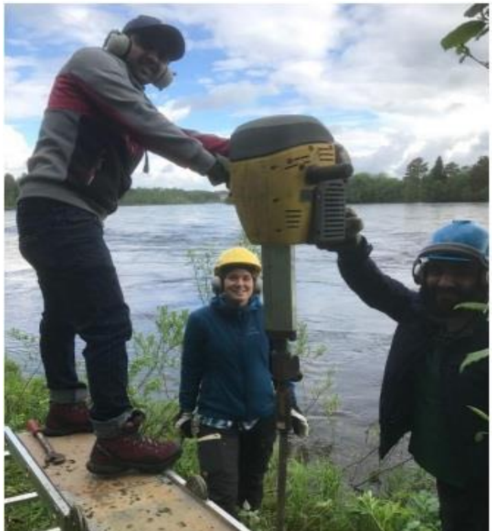
Figure 15 Sounding Test on Before Drilling Well
