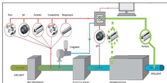
**Figure 1.** Concept of the TUO software-sensor. The sensor covered by dotted line indicates the proposed software-sensor
