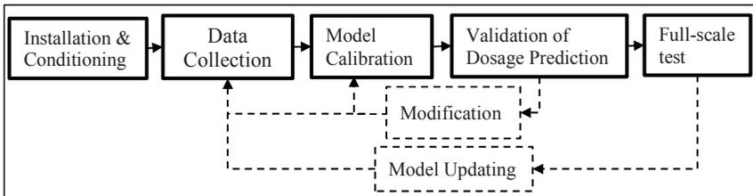
Figure 13. The procedure of full-scale tests. The solid line presents compulsory actions while the dotted line indicates non-compulsory actions
