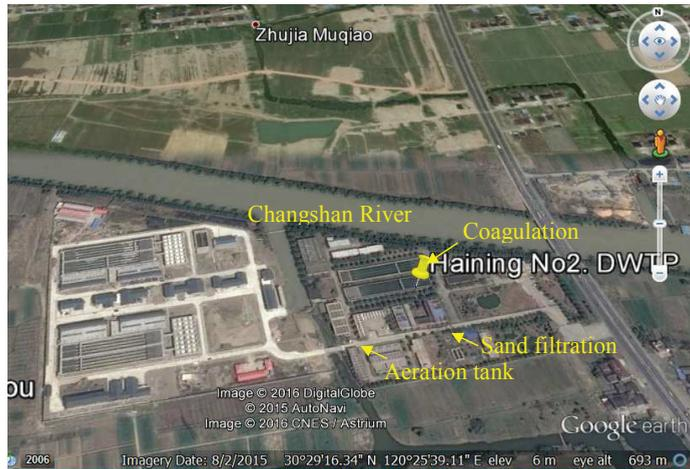
*Figure 2. Overview of Haining Number two DWT plant, Changshan River as water source, aeration tank, coagulation process and sand filtration are marked.*
