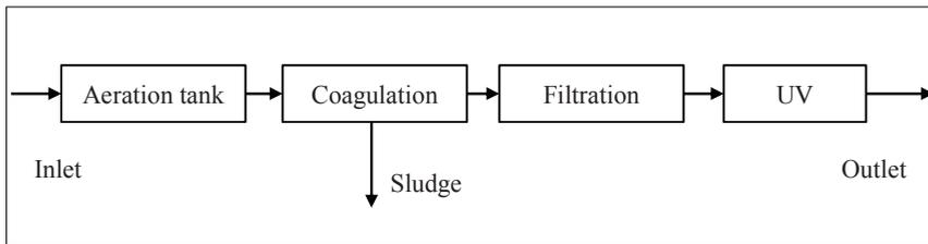
*Figure 6. Schematic of treatment process in SDWTP*
