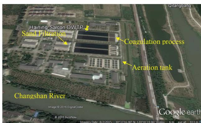
Figure 5. Overview of Haining Salcon DWT plant, Changshan River as water source, aeration tank, coagulation process and sand filtration are marked
