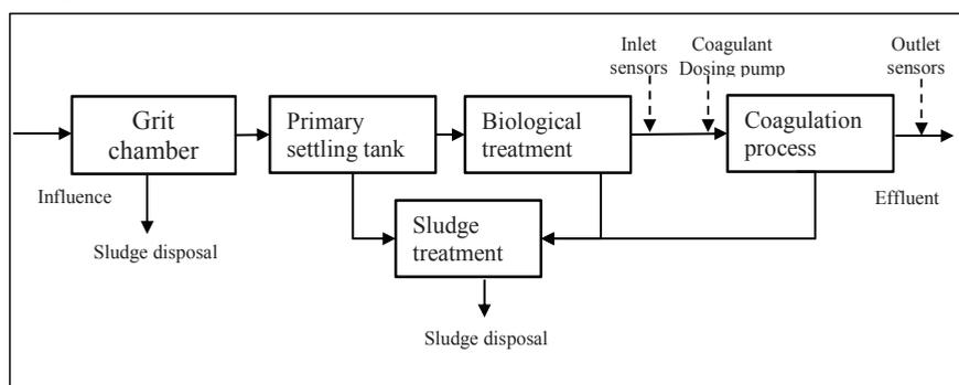
Figure 2, Schematic of treatment process in NRA WWTP, dash lines indicate the location of device and online sensors
