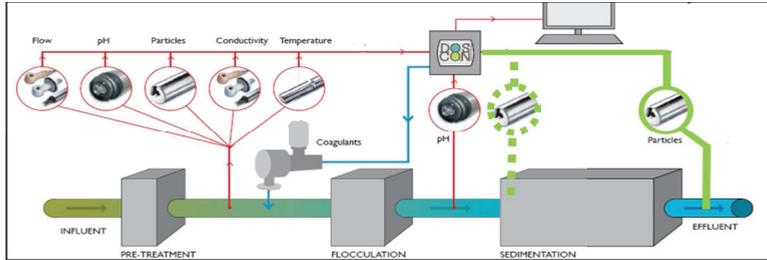
Figure 22. Concept of the TUO software-sensor (Instruments covered solid line present physical online sensors whereas the TUO software-sensor within the dotted line)
