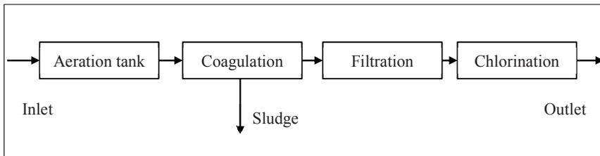
Figure 3. Schematic of treatment process in N2DWTP
