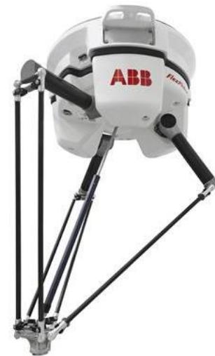
(b) The ABB's IRB 360 FlexPicker is a high speed robotic picking and packing technology. Courtesy of ABB.
