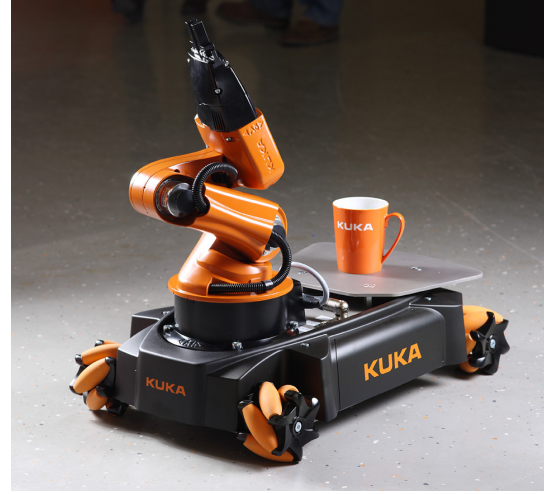
(b) The Kuka mobile manipulator consists of a five degree of freedom arm and an omnidirectional mobile platform. Courtesy of Kuka.
