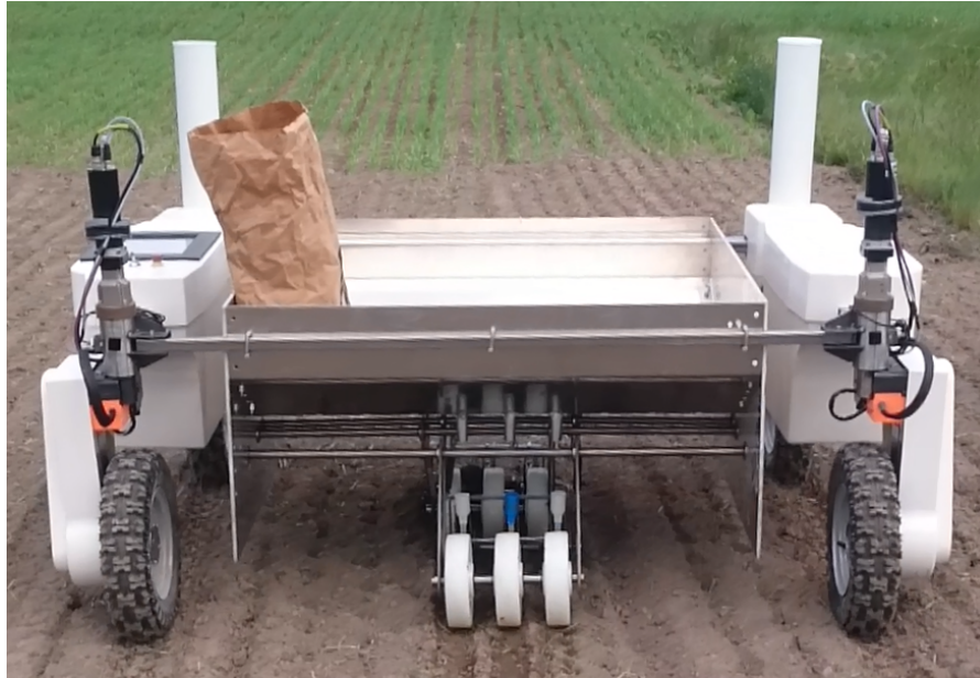
Figure 9.4: Thorvald with an early precision seeding tool prototype
