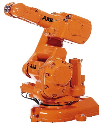
(b) The IRB 140 ABB serial manipulator is a six axes multipurpose industrial robot and handles a payload of 6kg with a reach of 810mm. Courtesy of ABB.
