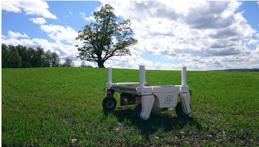
Figure 9.1: The Thorvald platform. Attached is an early prototype of a precision seeding tool.
