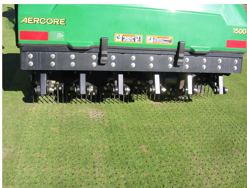
Photo 9. Spiking with 8 mm solid tines at Apelsvoll 27 Aug. 2007 (Photo: Tatsiana Espevig).
