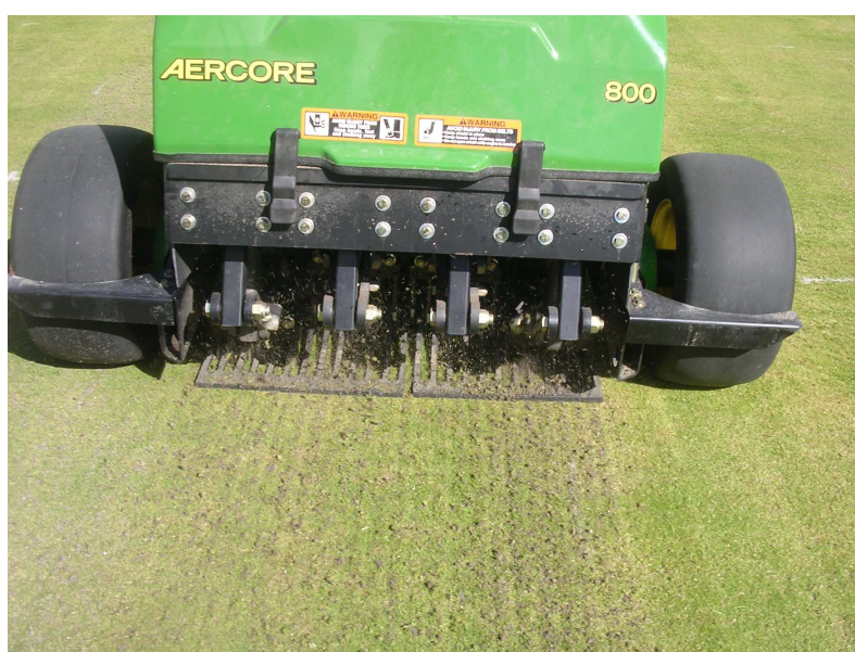
Photo 8. Coring with 6 mm hollow tines on approximately two months old velvet bentgrass green at Landvik, 31 July 2007 (Photo: Trygve S. Aamlid).
