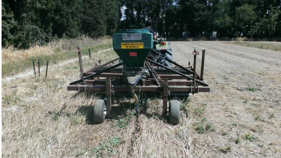
Picture 6: Soil strip tillage combined with fertilisation (06/06/2017)
