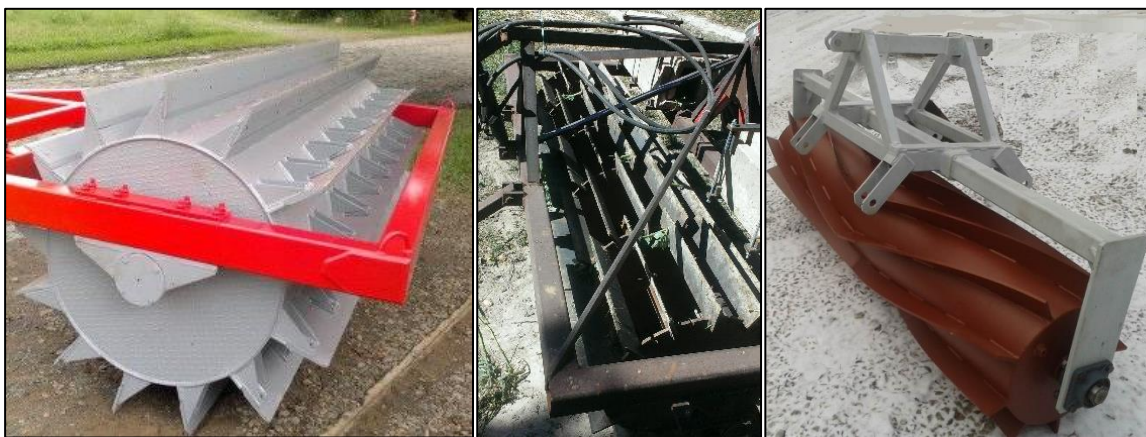
Figure 2: Different roller-crimper's blade type (from the left to the right: straight blades 5 , short-staggered straight blades 6 and spiral blades 7 )
