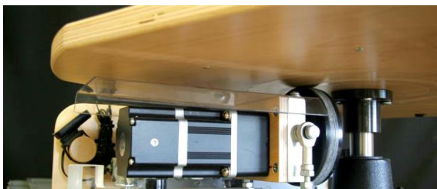
Figure 5-12. Example of the use of a drive wheel rotating the platform from underneath by friction
