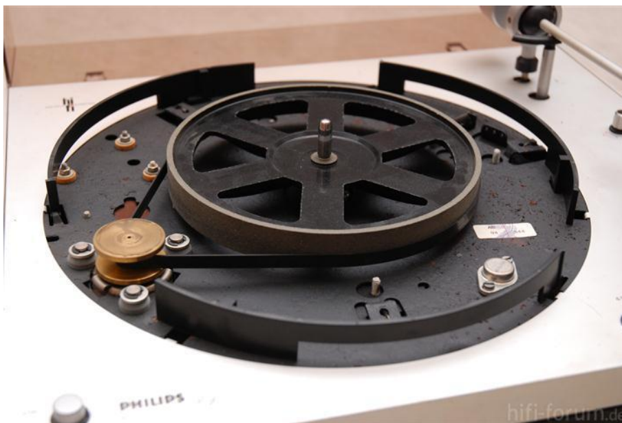
Figure 5-8. Example of the use of a flat belt drive in a Philips turntable [56]
