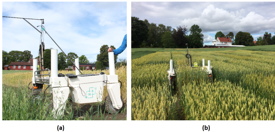
FIG. 3.6: Thorvald with (a) the rig for camera attachment shown (before attaching sensor and camera) and (b) in the midst of both the wheat and the process of photographing.
